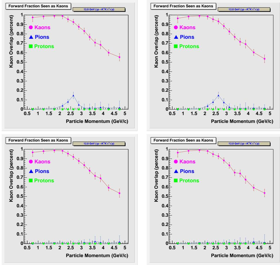
Figure 7: The fraction of  $K$ 's,  $\pi$ 's and  $p$ 's which are identified as  $K$ 's as a function of particle momentum. The plots use mass window 6 and the Čerenkov system with  $n = 1.0014$ . The upper left figure has no segmentation and  $n = 1.0014$ . The upper right figure has six segments with  $n = 1.0014$ . The upper right figure has one segment with  $n = 1.0024$ . The upper right figure has six segments with  $n = 1.0024$ .
