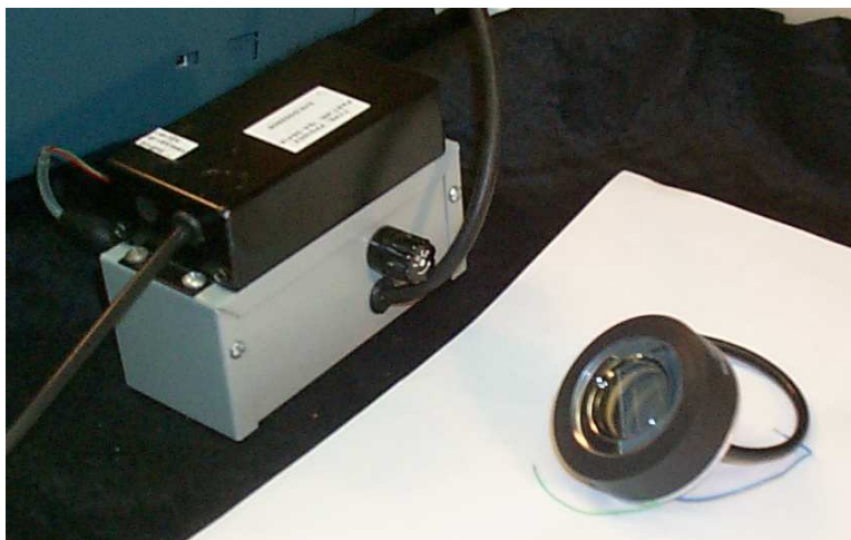
Figure 1: The PP0350G HPD (right) showing its overall size as well as its active area (innermost circle – photo-cathode window). Also displayed are the PP0100Z HV power supply (black box) and its custom-built voltage distributor (gray box).
