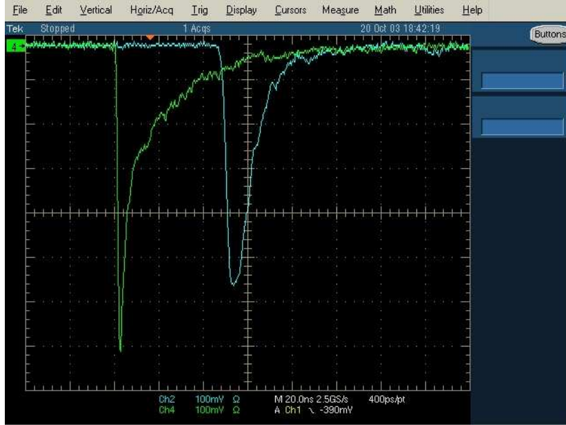
FIG. 4: The shape of pulses from SiPM and PMT. A light flasher (OPTITRON) was used as a light source. The green and blue lines are signals from SiPM and PMT, respectively. The high voltage for the PMT was 1900V and the bias for the SiPM was 55.5 V.
