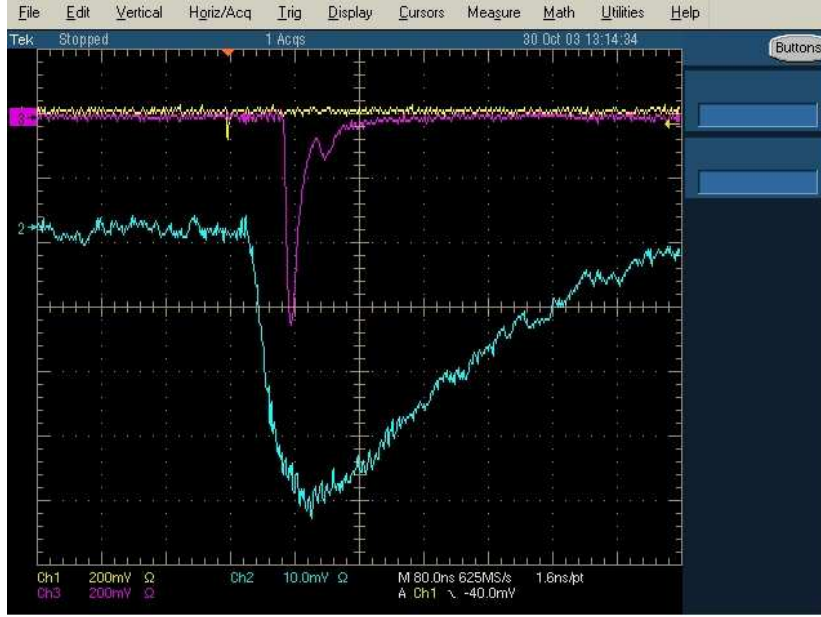
FIG. 2: A picture of a typical signal from a HPD with an OPA preamplifier. The yellow line (channel 1) corresponds to the triggering signal, the blue line (channel 2) is the signal from the HPD + preamplifier and the red line (channel 3) is the signal from a PMT.
