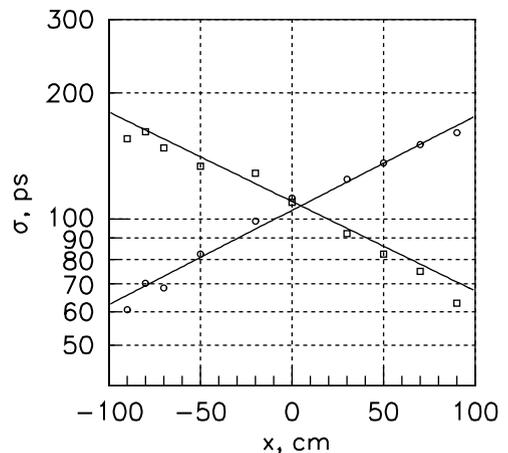
Fig. 9. Time resolution vs.  $x$  after correction for time-walk effect.
