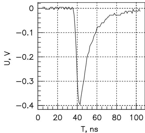
Fig. 2. Signal shape after 40 m cable measured at the center of scintillation bar with Tektronix 724D digital oscilloscope.
