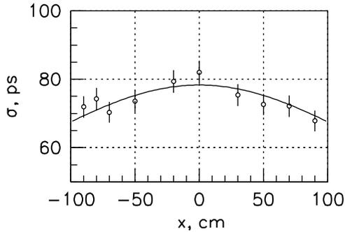
Fig. 10. The  $x$ -dependence of time resolution for B1 after time-walk correction. Solid line represents the equation (2) with  $\sigma_b = 74$  ps,  $\lambda_b = 124$  cm.
