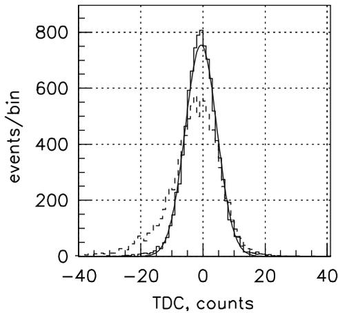
Fig. 6. Time spectra measured with LED: dashed histogram—raw spectrum; solid histogram—spectrum after correction for time-walk effect; solid line—Gaussian fit.
