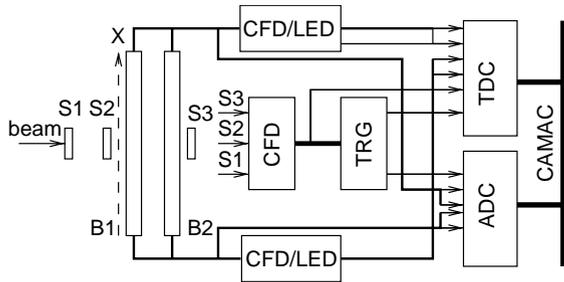
Fig. 1. Experimental setup and block diagram of electronics: S1–S3—beam counters; B1, B2—TOF counters; CFD, LED—constant fraction and leading edge discriminators; TRG—coincidence unit.
