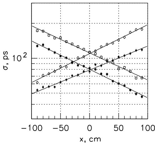
Fig. 4. Time resolution of PMT signals vs.  $x$  measured with CFD for perpendicular (open symbols) and parallel (closed symbols) position of B1 (see text).
