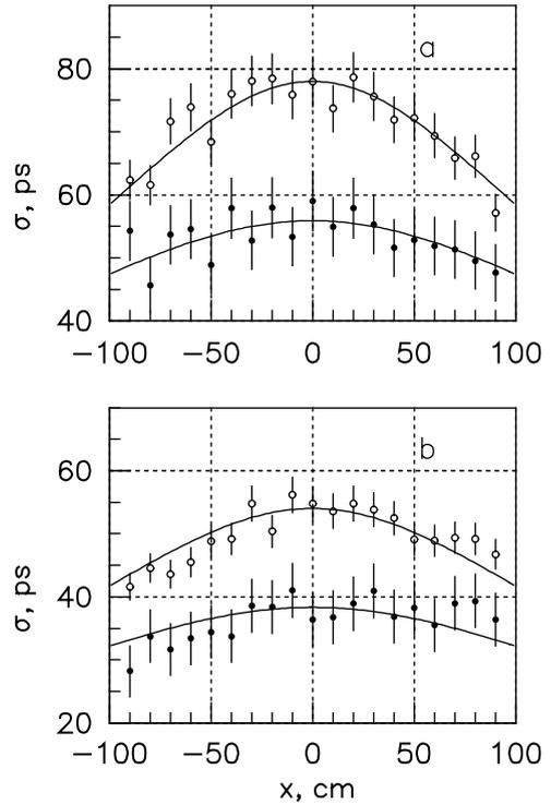
Fig. 5. The time resolution of B1 (open symbols) and B1 + B2 (closed symbols) for perpendicular (a) and parallel (b) positions of the bars.
