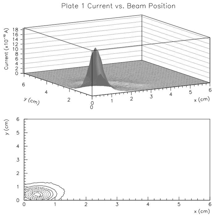
FIG. 2: Graphs of plate current versus  $x$  and  $y$  beam position for plates one and five. The information from these graphs was used to determine beam position from plate current in the final test of TPCD performance.
