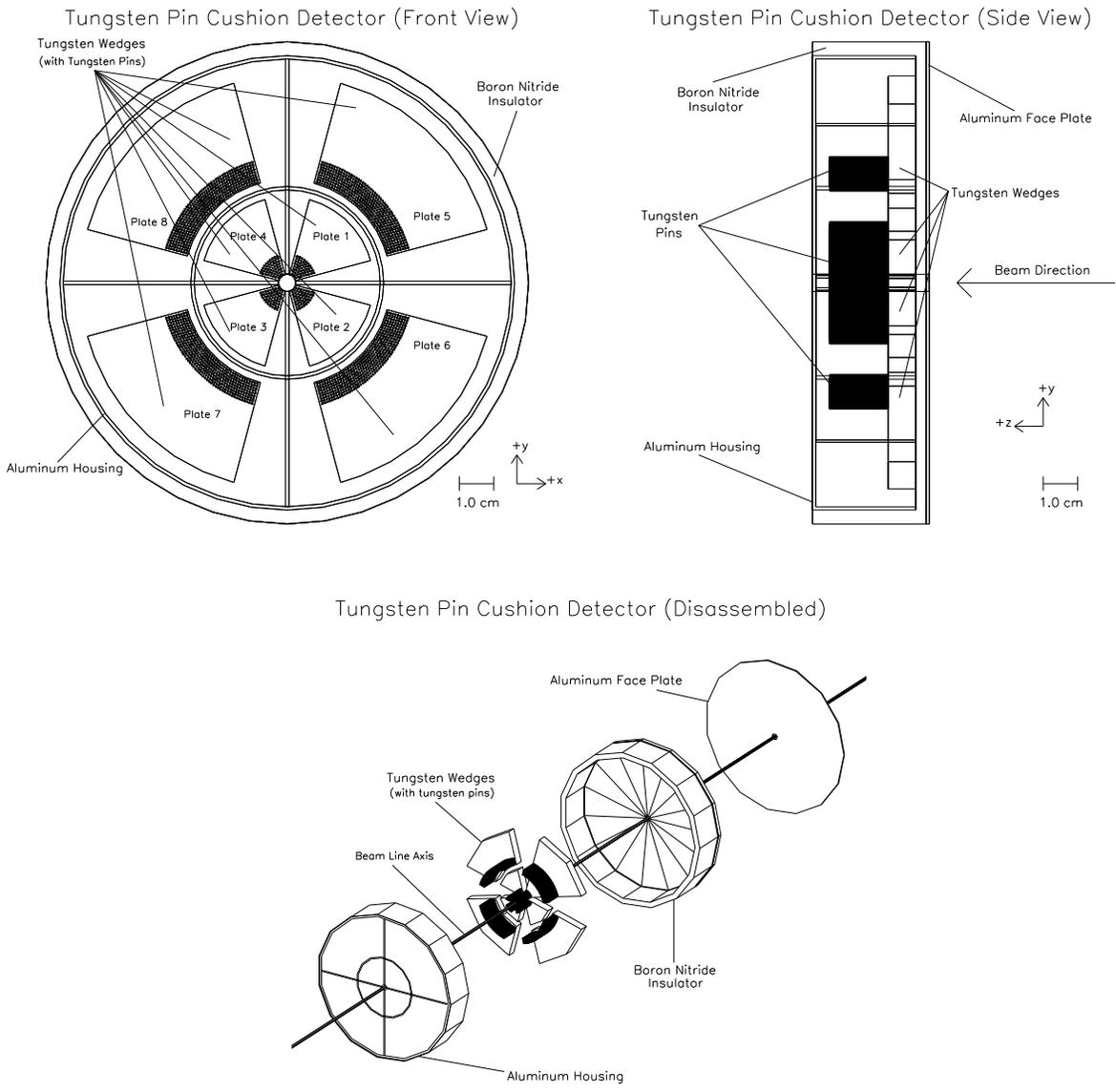
FIG. 1: Different views of the tungsten pin cushion detector. Note that the front view shows what number refers to what plate.
