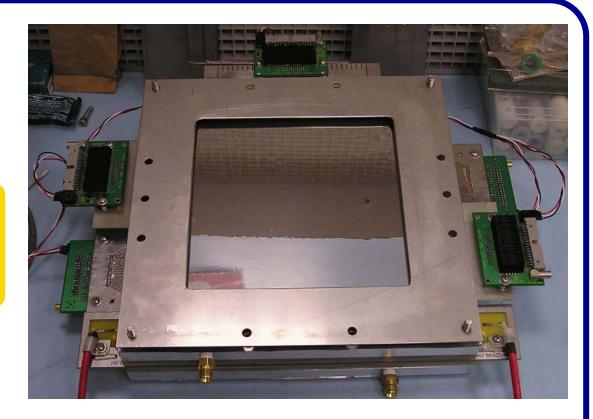
• 1 anode plane consisting of 16 sense wires (10 mm separation) Second configuration with alternating anode and field wires.
