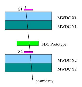
Trigger: coincidence between top and bottom scintillator paddles.
