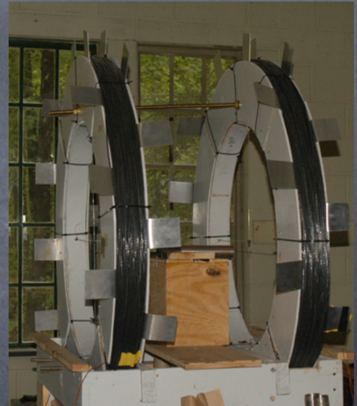
Helmholtz coils (200 G max) for shielding studies
