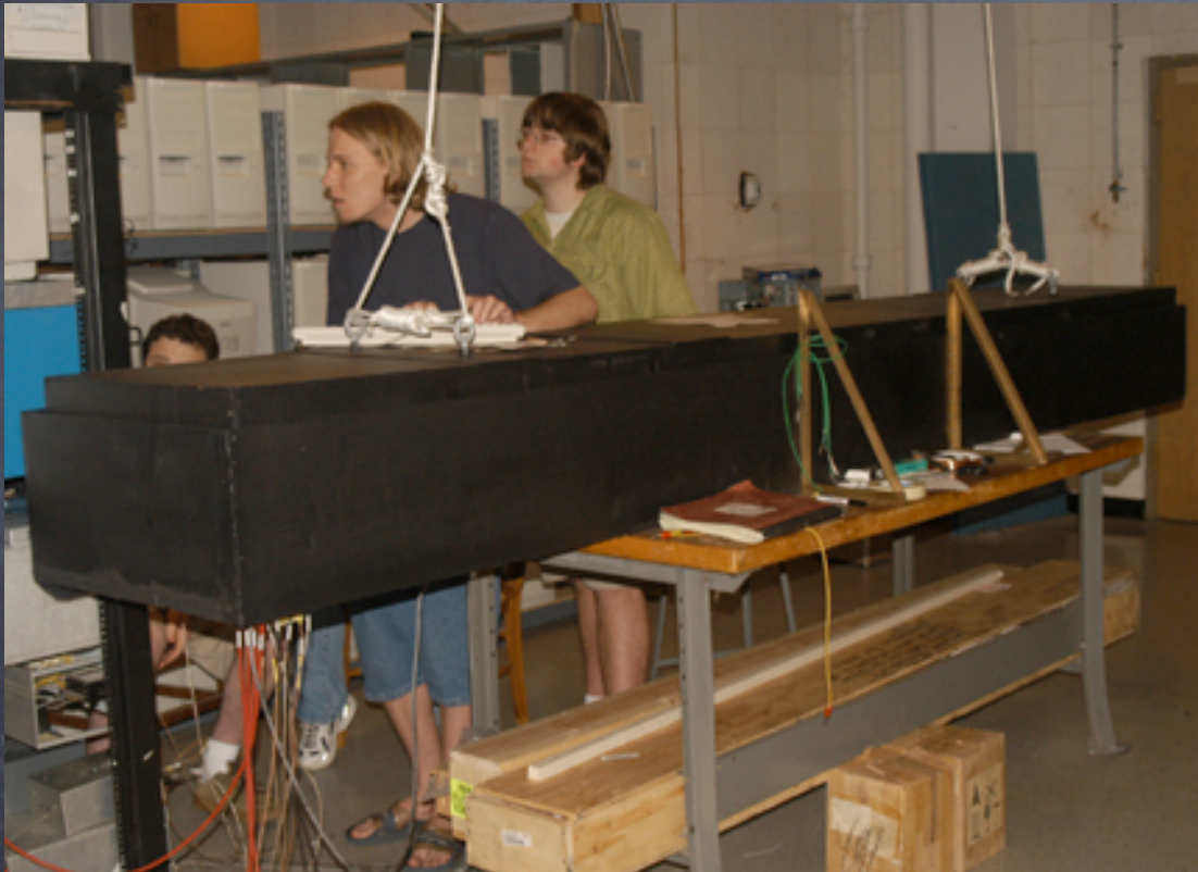
Black box for testing 2-m bars using cosmic rays
