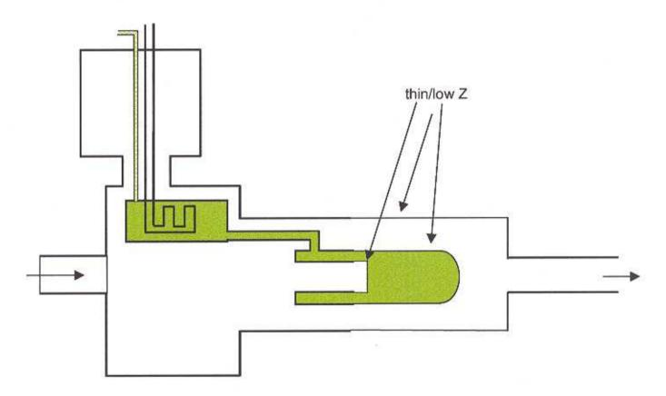
Mechanism to introduce solid target(s) - minimize blocking detector acceptance
