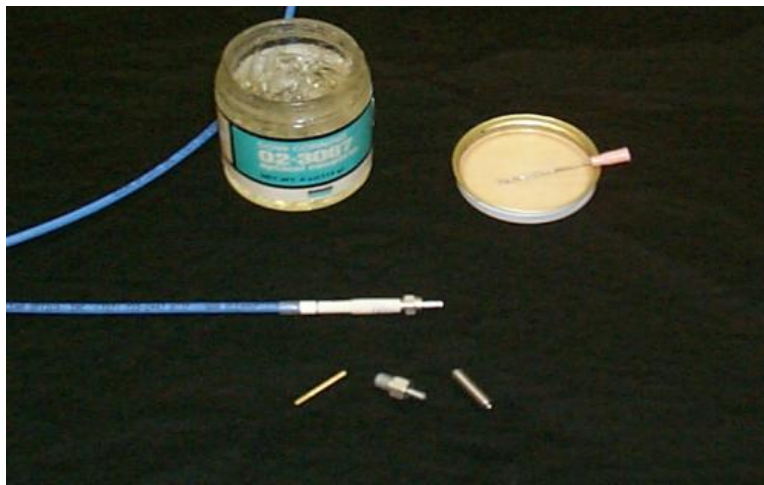
Figure 6: New connector disassembled, showing optical couplant and syringe tip used for the coupling
