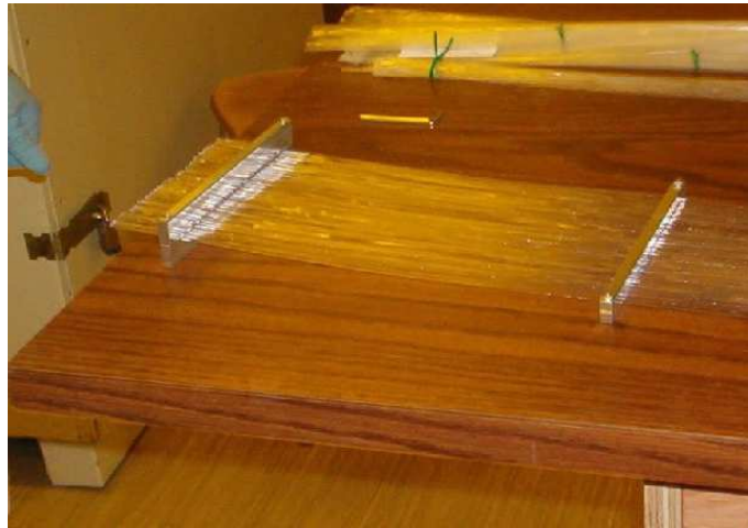
FIG. 7: Bundle of fibers after clamp and guide have been positioned.
