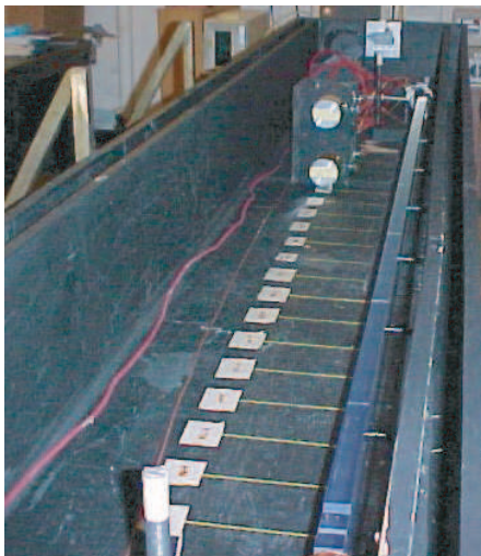
Figure 4.61: Part of the cosmic ray test facility showing a light-tight box inside of which is a 2-m long scintillator bar, read out at both ends, as well as a trigger telescope with two small scintillation counters that can be positioned along the bar.
