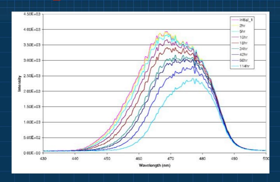
Controlled exposure to fluorescent lighting; LED 470nm, transmission spectrum
