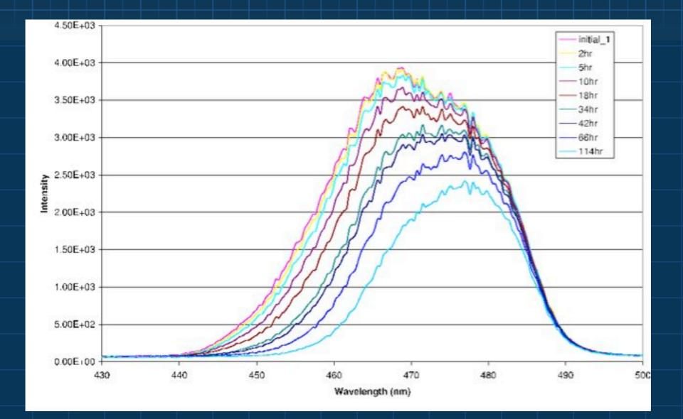
Controlled exposure to fluorescent lighting; LED 470nm, transmission spectrum
