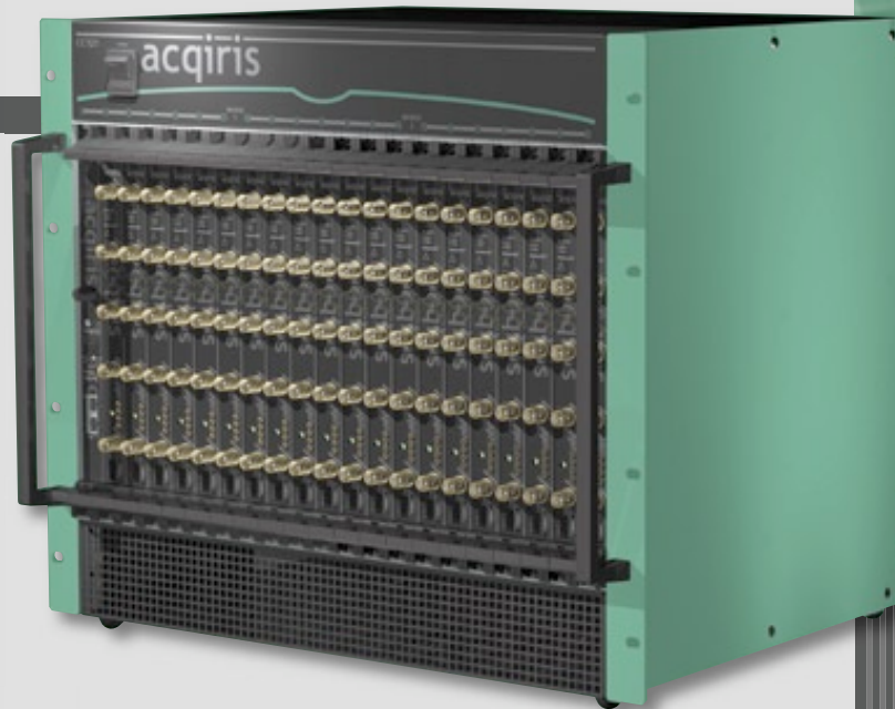
CC121 equipped with 20 1-4 GS/s quad-channel Digitizers (DC271) and one PCI interface for easy connection to a benchtop PC
