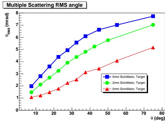
Figure 4: RMS value of the multiple scattering angles between the particle trajectory at the vertex and after passing through the target and the start counter.
