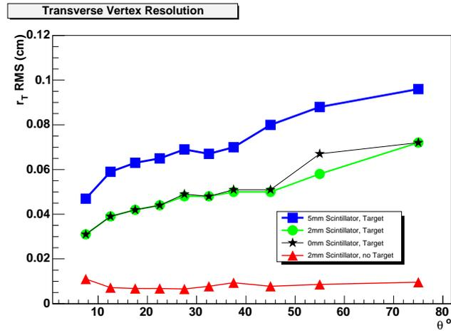
Figure 3: Transverse resolution (RMS value) of the reconstructed vertex.
