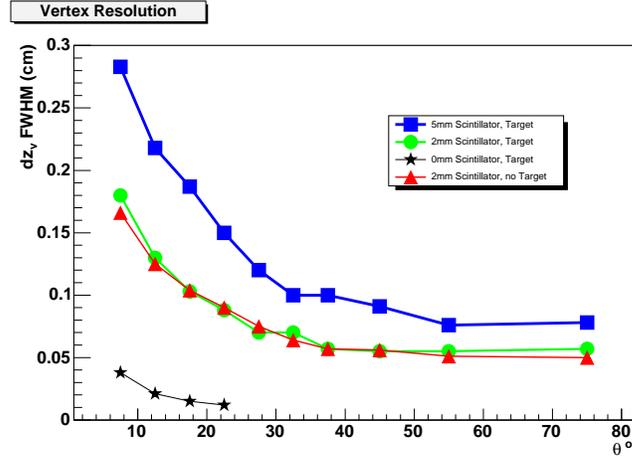
Figure 2: Width (FWHM) of the distribution of the difference between reconstructed ( $z_v^r$ ) and actual vertex position ( $z_v$ ).
