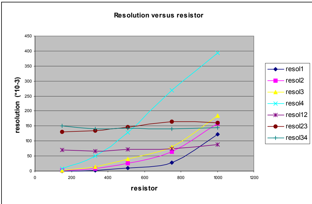
Figure 19: resolutions versus the R1 resistor
