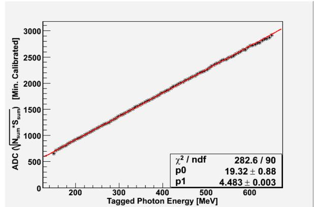
Fig. 7. A plot of the ADC geometric mean (minimization calibration) vs. tagger energy with a linear fit.
