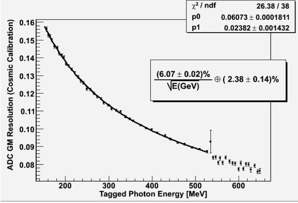
Fig. 11. The energy resolution using cosmic ray calibration for each cell
