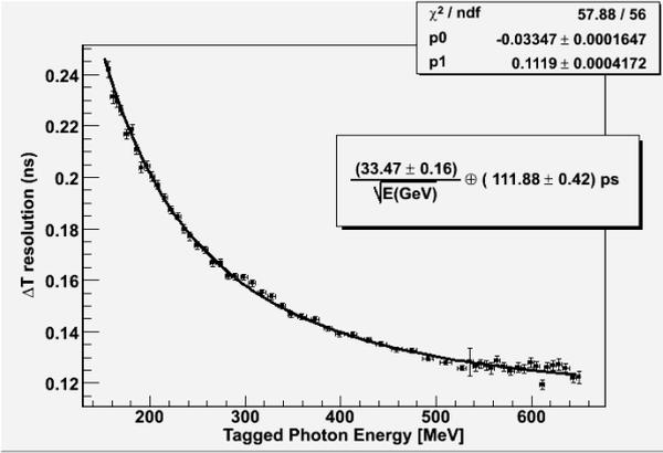
Fig. 23. The time difference resolution,  $\sigma_{\Delta T}$ , as a function of energy.
