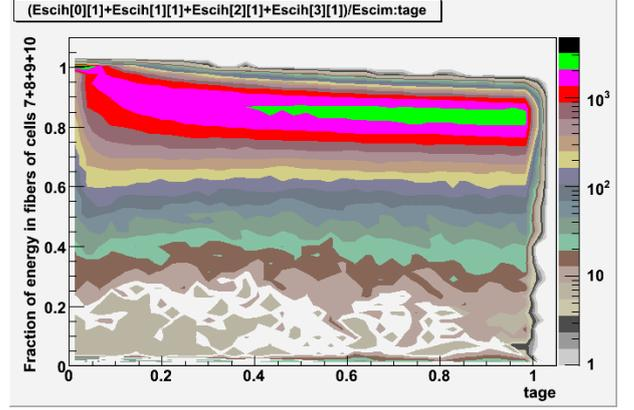
Fig. 21. From Monte Carlo: The fraction of energy deposited in the fibres of cells 7,8,9 and 10.
