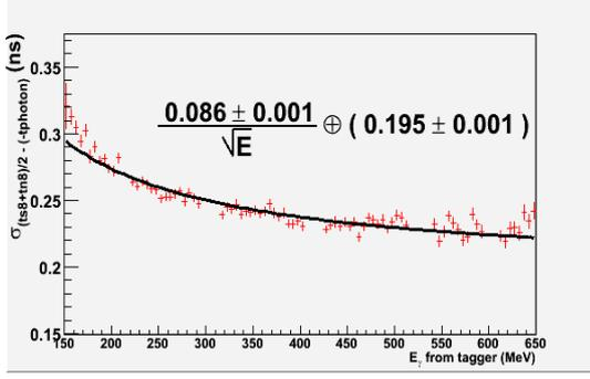
Fig. 20. Timing resolution from fitting the slices of Figure 18
