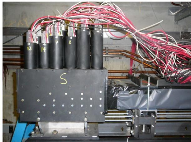
Fig. 3. The black box encloses the 18 light guides and PMTs with cables attached for the South end of the BCAL module and is similar to the North end. The BCAL Pb/Sci-Fi matrix is wrapped in Teflar on the right and pressed against the light guides coupled with a silicone cookie.
