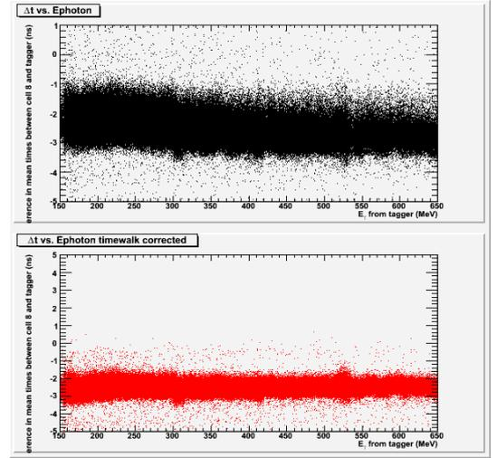
Fig. 18.  $(tn8+ts8)/2 - (-tphoton)$  vs. Tagger Energy (MeV for Cell 8). The top plot is before time walk corrections. The bottom plot is after walk corrections.
