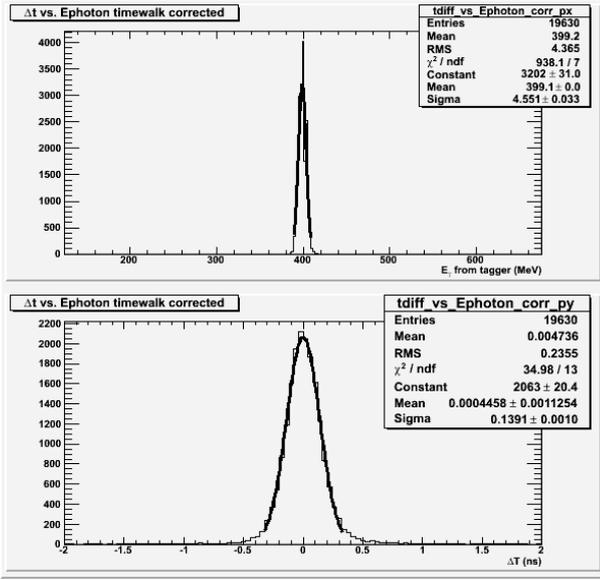
Fig. 22. An example of the time difference distribution for t-counter 28
