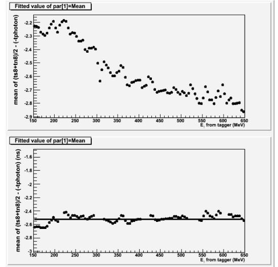
Fig. 19. The mean of the distribution in Figure 18 The top plot is before time walk corrections. The bottom plot is after corrections.
