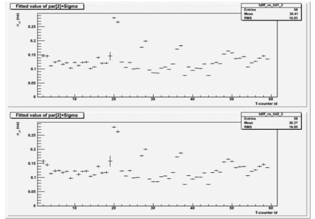
Fig. 25. The resolution of the time difference between adjacent t-counters of the Hall-B tagger.
