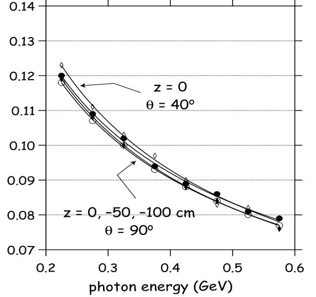
Fig. 10. The energy resolution for three z-positions.
