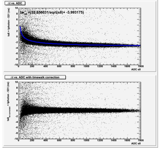
Fig. 14. ADC vs. TDC for cell South 8. The uncorrected time walk is seen in the top plot. The bottom plot shows the corrected time.
