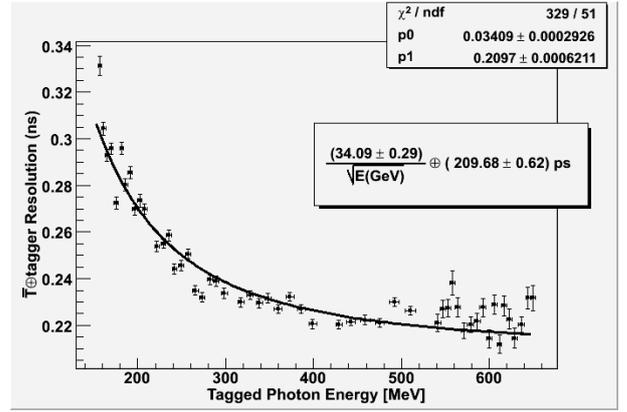
Fig. 24. The mean time resolution,  $\sigma_{\bar{T}}$ , without the tagger resolution extracted.
