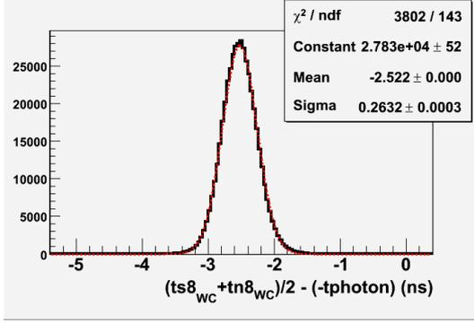
Fig. 16. The mean timer distribution of cell 8 corrected for time walk and referenced with the tagger
