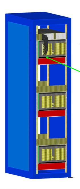
'Fill' View 3 crates per rack 256 'channels' per crate (768 'channels' per rack)
