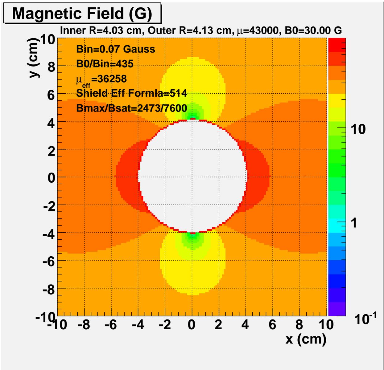
Figure 4: Plots of the total magnetic flux density in a 3.25 in. diameter shield. The unperturbed magnetic field is 30 G in the x-direction. The maximum field in the  $\mu$ -metal shield is 2473 G below the saturation value of 7600 G. The shield effectiveness is 515 and results in a magnetic field inside the shield of about 0.06 G. This value is to be compared to a measured value of 0.22 G [?].
