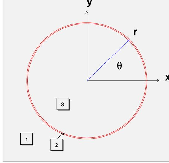
Figure 1: Geometry and coordinate system for calculation. The axis of the magnetic shield is oriented along the  $z$ -axis. The three regions are indicated by the boxes: region 1 outside the shield, region 2 in the  $\mu$ -metal shield itself, and region 3 constituting the area inside the shield.
