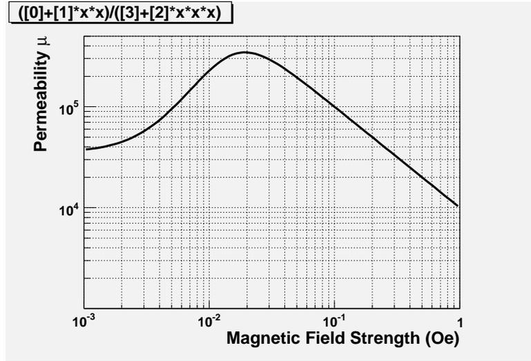
Figure 2: Parameterization of the permeability of typical high permeability material, such as AD-MU-78, as a function of the magnetic field strength.
