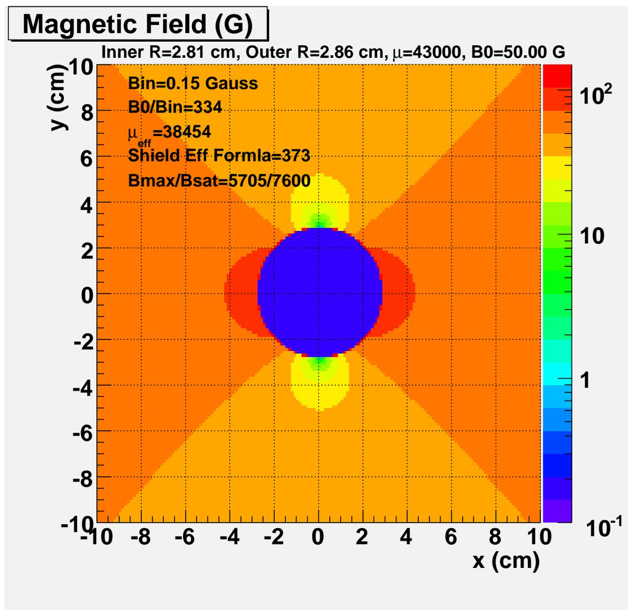
Figure 10: Plots of the total magnetic flux density. The unperturbed magnetic field is 50 G in the x-direction. The maximum field in the  $\mu$ -metal shield is 5705 G, close to the saturation value of 7600 G. The shield effectiveness is 334 and results in a magnetic field inside the shield of about 0.15 G.
