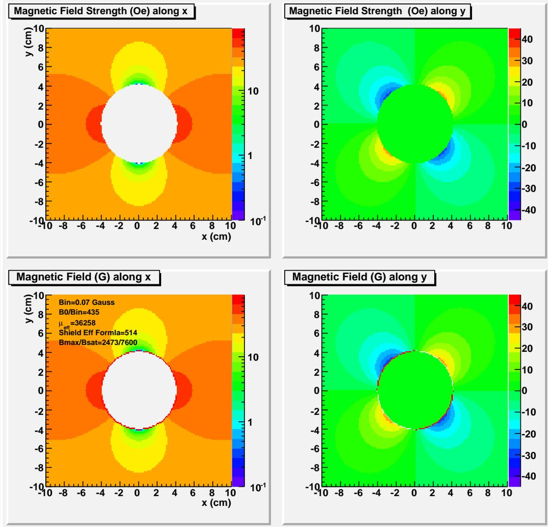
Figure 3: Plots of the magnetic field strength (top) and magnetic flux density (bottom) along the x and y-axis inside a 3.25 in. diameter shield. The unperturbed magnetic field is 30 G in the x-direction.
