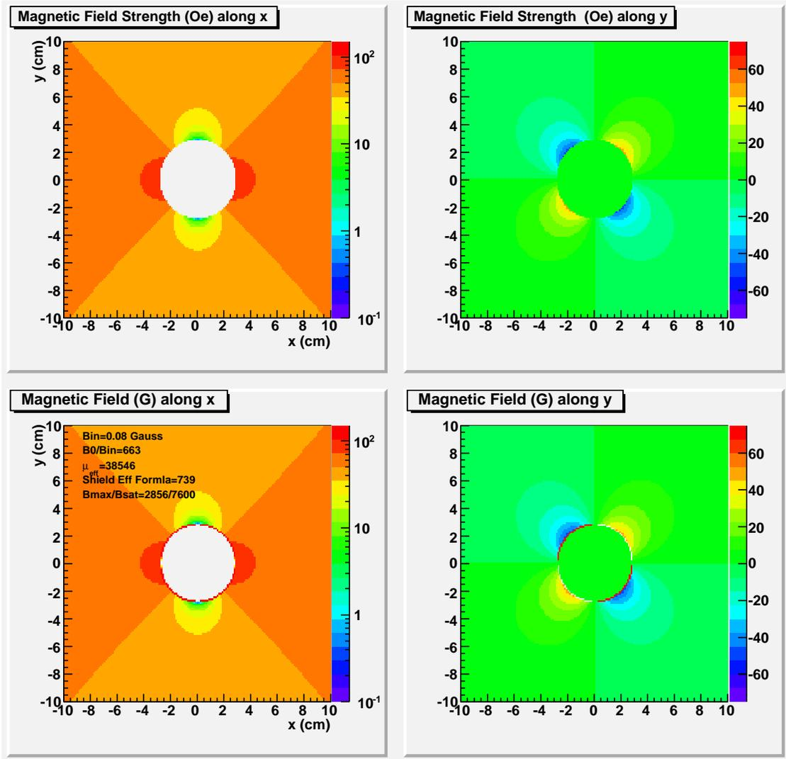
Figure 5: Plots of the magnetic field strength (top) and magnetic flux density (bottom) along the x and y-axis. The unperturbed magnetic field is 50 G in the x-direction.
