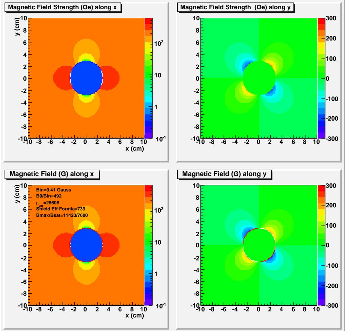
Figure 7: Plots of the magnetic field strength (top) and magnetic flux density (bottom) along the x and y-axis. The unperturbed magnetic field is 200 G in the x-direction.
