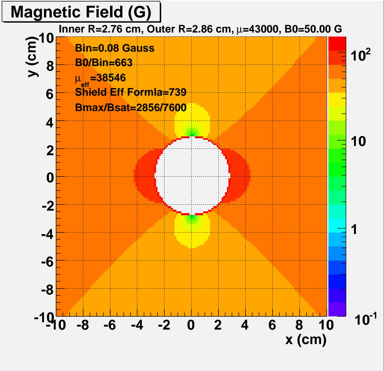
Figure 6: Plots of the total magnetic flux density. The unperturbed magnetic field is 50 G in the x-direction. The maximum field in the  $\mu$ -metal shield is 2856 G, well below the saturation value of 7600 G. The shield effectiveness is 740 and results in a magnetic field inside the shield of less than 0.1 G.
