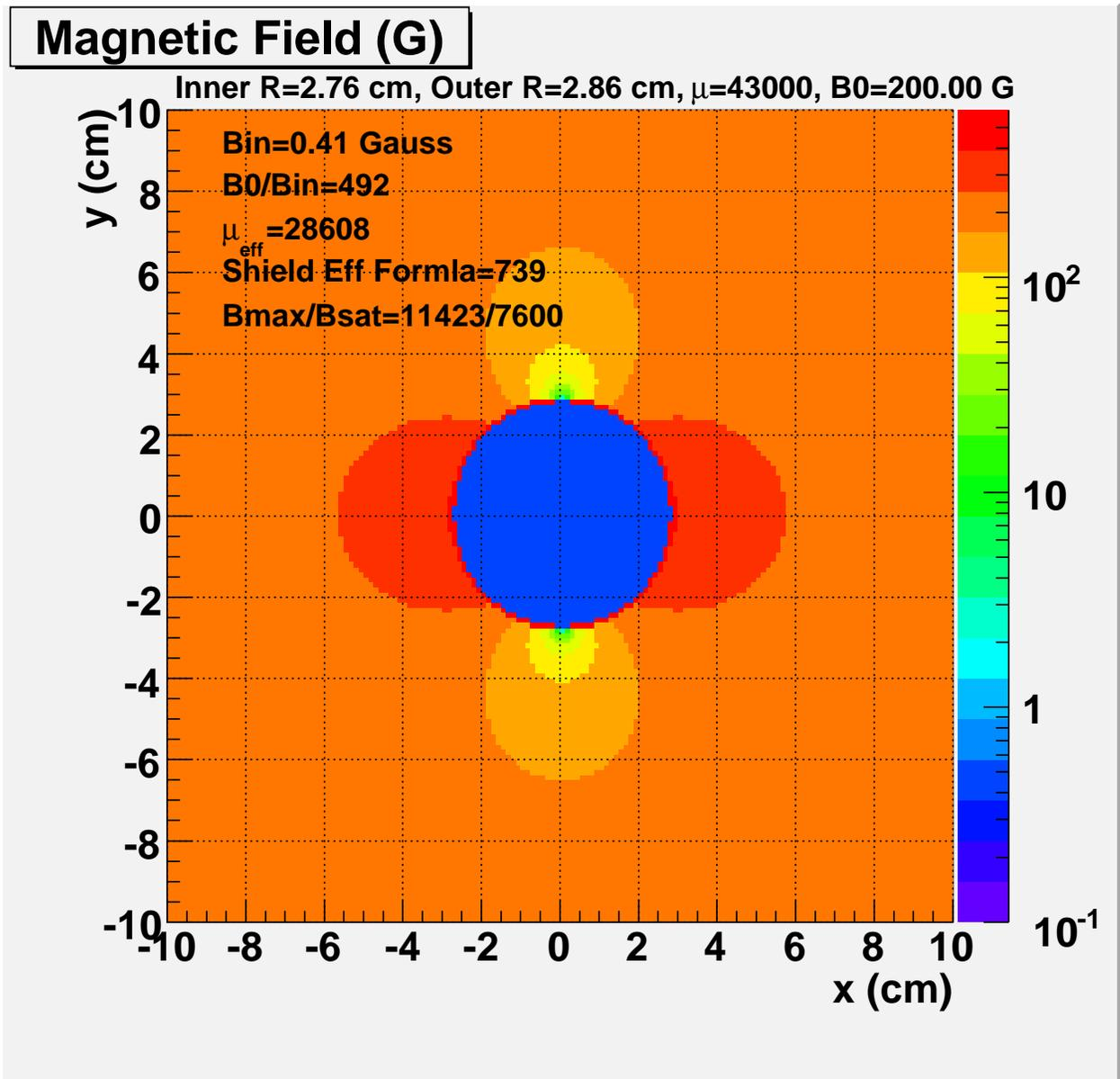
Figure 8: Plots of the total magnetic flux density. The unperturbed magnetic field is 200 G in the x-direction. The maximum field in the  $\mu$ -metal shield is 11423 G above the saturation value of 7600 G. The shield effectiveness is 492 and results in a magnetic field inside the shield of about 0.4 G.
