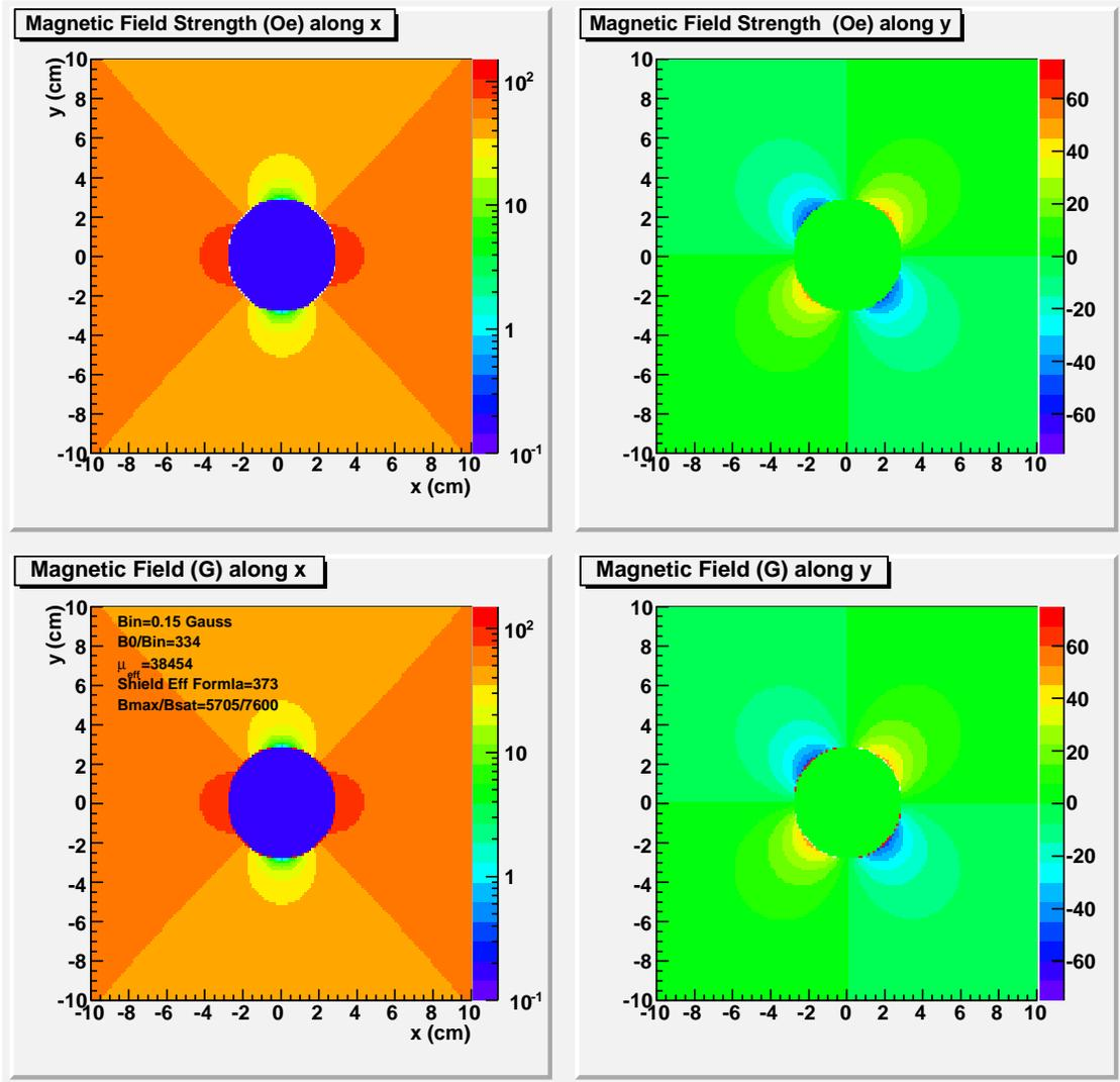
Figure 9: Plots of the magnetic field strength (top) and magnetic flux density (bottom) along the x and y-axis. The unperturbed magnetic field is 50 G in the x-direction.
