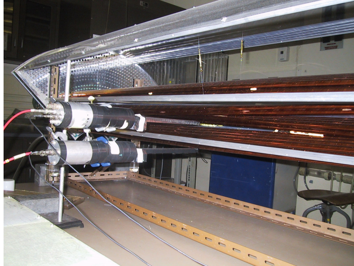
Figure 18: A photograph of the 2 m long CDC prototype at Carnegie Mellon. The copper-colored tubes are kapton and the silver-colored ones are mylar. Also shown are a pair of small scintillators used in a specialized cosmic trigger.
