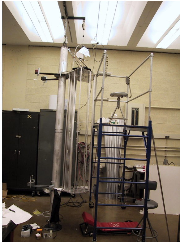
Figure 16: The CDC prototype in its vertical position while straw tubes are installed and wires are strung.
