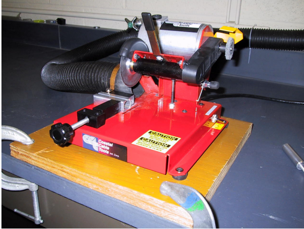
Figure 14: The high-speed saw used to cut the CDC straw tubes to the appropriate length. The black knob on the left-side of the saw tightens a clamp that holds the tubes in place for cutting. The right-hand picture shows a mylar straw being cut by the saw.
