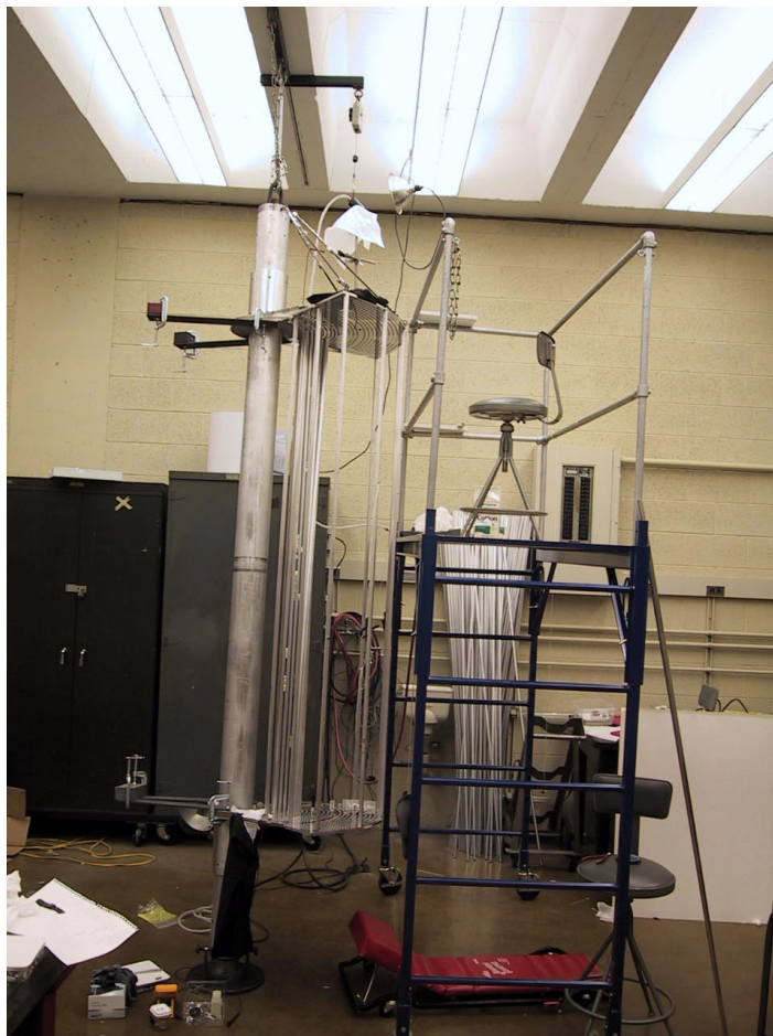
Figure 18: The CDC prototype in its vertical position while straw tubes are installed and wires are strung.
