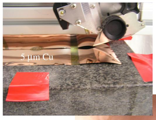
All 5 µm Cu and 2 µm Cu prototype boards on hand have been successfully trimmed!
