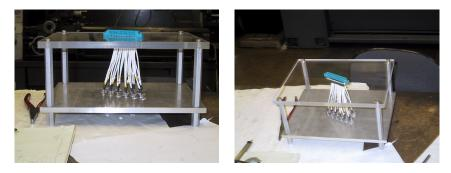
In this design, a gas-tight connector is made. The wires are up to about 12cm long and are attached to the chamber wires by reaching in from the side.
