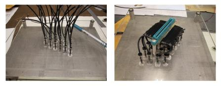
In this design, a gas-tight connection is made around the coaxial cable. We are still checking this. The wires are up to about 9cm long and are attached to the chamber wires pushing through a
