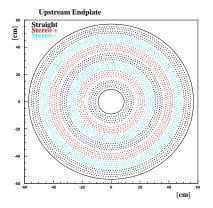
The hole pattern on the up-stream end plate,  $a \rightarrow a = a$
