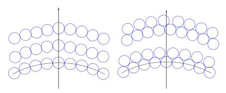
Wire layouts in the two designs. Left is the original design with the open-pack geometry. Right is the new design with the close-pack geometry.
