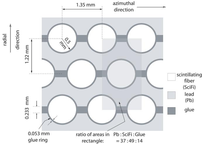
Fig. 1. A close up of the lead matrix is shown.
