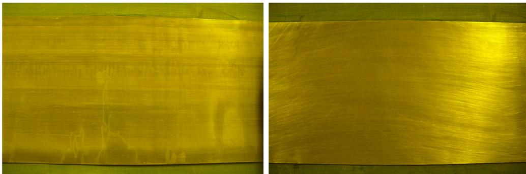
Fig. 3. Photographs of a lead sample before (left) and after (right) scrubbing and cleaning. The removal of discoloration is visible near the bottom quarter strip of the sheet.
