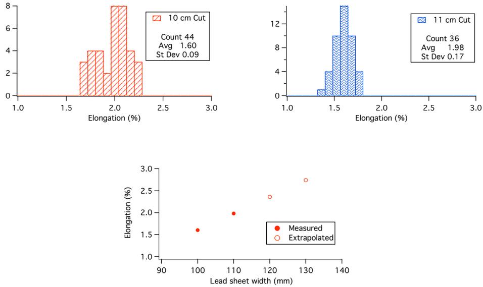
Fig. 5. Histogram of the percent elongation of the lead for the 10-cm (top left) and 11 cm (top right) cuts. The average elongation is plotted versus the lead sheet width/cut (bottom) assuming a linear behaviour. Details are provided in the text.
