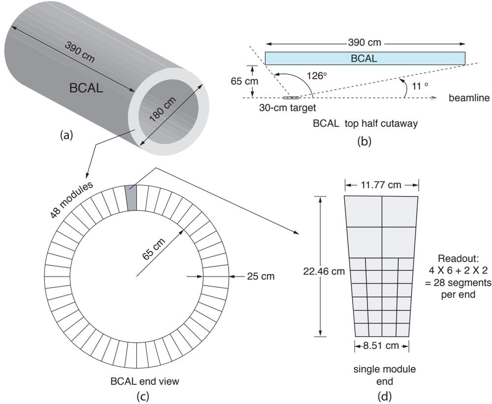
Fig. 2. The GlueX BCAL calorimeter. (a) overall schematic; (b) top-half cutaway showing the placement of BCAL with respect to the beamline and liquid hydrogen target; (c) end view showing 48 modules; and (d) end view of a module showing readout segmentation.
