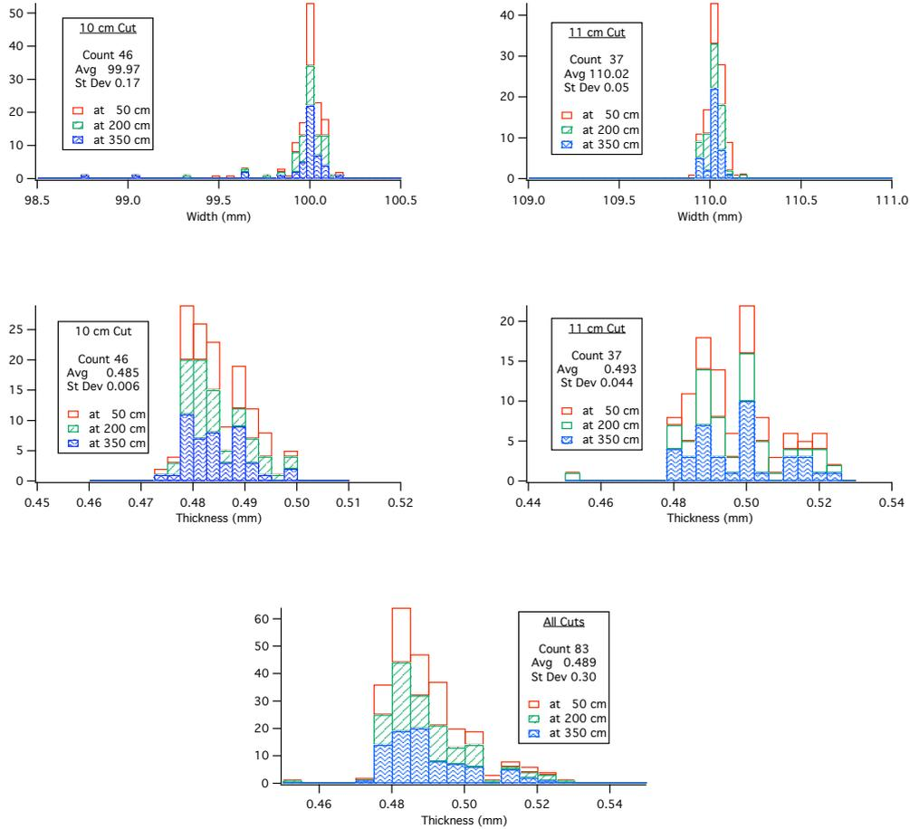
Fig. 4. The Regina histograms of lead width and thickness based on the two width cuts. Measurements were taken near the edge of each cut at approximately 50 cm, 200 cm and 350 cm from one cut end. The bottom panel combines the thickness measurements for both cuts.
