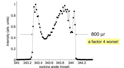
Test of #3: decouple/damp goniometer vibration using a "soft mount" (wax)
