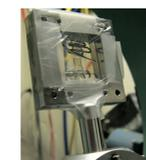
Loading the wires with extra mass shifts down the frequencies of the fundamental resonances.
