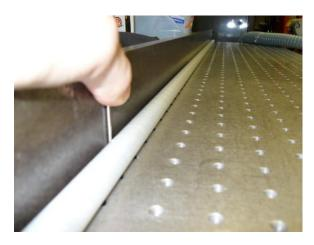
4. Allow the tube to fall slowly through the 0.7" aperture in the donut onto a pad on the floor. If the cross section of the tube is oval at any point, the tube will stick in the aperture. Reject the tube if gravity (and a small amount of wiggling to make sure it is not something about the angle of the donut) is not sufficient to make the tube fall through.
