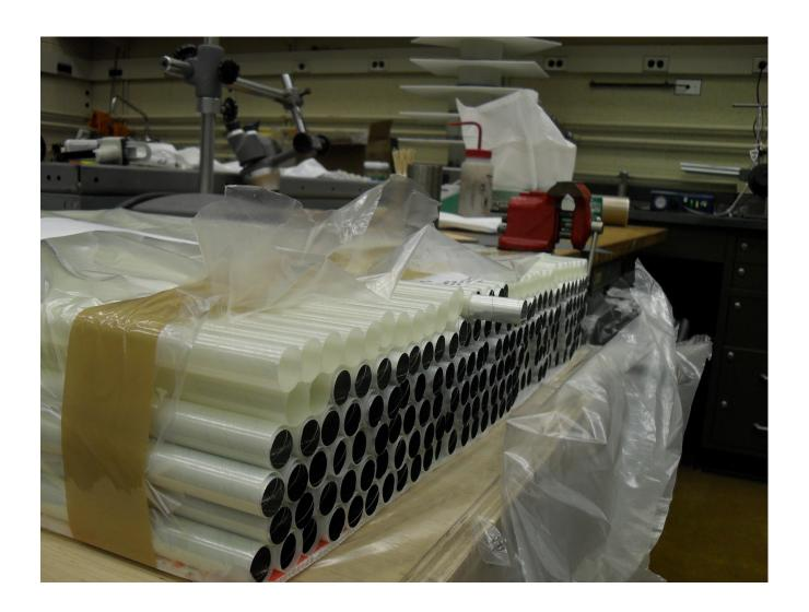
1. Visually inspect each tube thoroughly making sure there are no blemishes such as glue spots or dents. If there are, circle them with a permanent marker so that they can be easily spotted during future inspections, and put them in the rejection box.
