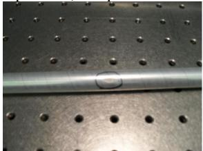
2. Roll the tube across a clean, flat table to make sure it is completely cylindrical. If the tube favors one side by rolling to a certain position, reject it.
