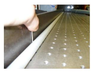
4. Allow the tube to fall slowly through the 0.625" aperture in the donut onto a pad on the floor. If the cross section of the tube is oval at any point, the tube will stick in the aperture. Reject the tube if gravity (and a small amount of wiggling to make sure it is not something about the angle of the donut) is not sufficient to make the tube fall through.
