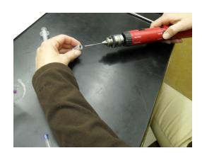
The needle should slide in about 1/8" and then out easily. If it does, the ports are ok.
