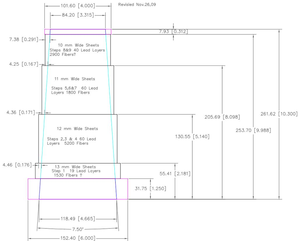
Fig. 4. The BCAL design dimensions are shown, including the base (outer) and top (inner) plates. The “Mayan” pyramid shape adopted during construction is shown in green, whereas the tapered blue lines display the final machined dimensions. *Note that this figure can be viewed and/or printed using Adobe products (Acrobat Reader, Acrobat Pro). It is not visible using the Mac OS X Preview application.*
