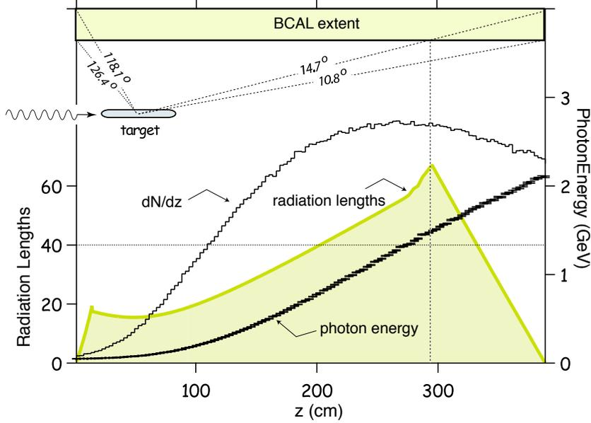
Fig. 2. The distribution of photons, their energy and integrated path length through the Pb/SciFi matrix as a function of position along the length of the BCAL for one of the GLUEX signature reactions,  $\gamma p \rightarrow \eta \pi^0 p \rightarrow 4\gamma p$ , is shown. The target position and angular range subtended by the BCAL are also presented. (Courtesy of Alex Dzierba.)
