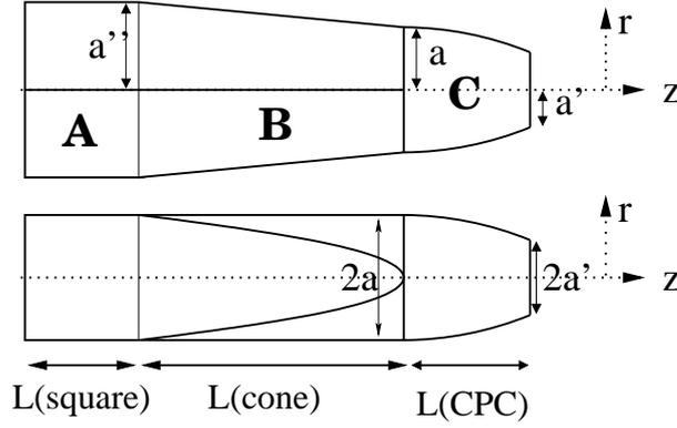
Fig. 5. A schematic drawing of the light collectors [9]. The total length (square plus cone plus CPC) is 10 cm.
