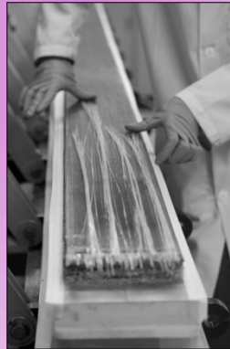
Optical epoxy is used to adhere the fibres to the lead sheets in the matrix. Each fibre corresponds to a groove in the lead sheets below and above the layer of fibres.
