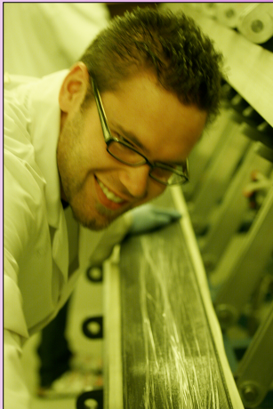
Optical epoxy is used to adhere the fibres to the lead sheets in the matrix. Each fibre corresponds to a groove in the lead sheets below and above the layer of fibres.
