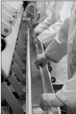
Each layer of the matrix consists of two layers of optical epoxy, one layer of fibres, and one sheet of lead.
