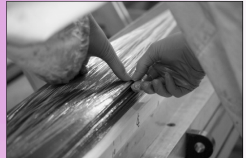
Fibres are counted and bundled according to the width of the layer. Each bundle is carefully laid onto the epoxy covered matrix, and each fibre is pushed into a separate groove.
