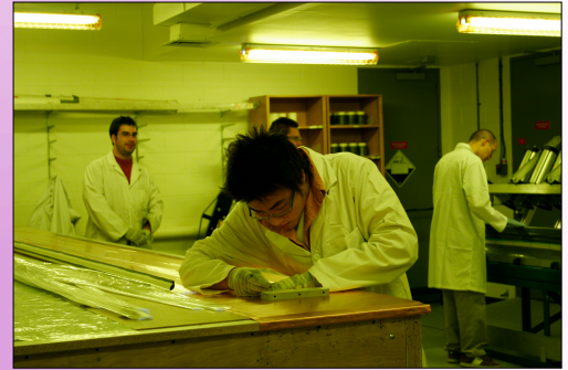
Fibres are counted and bundled according to the width of the layer. Each bundle is carefully laid onto the epoxy covered matrix, and each fibre is pushed into a separate groove.
