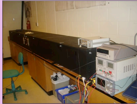
Fibres arrive packaged, boxed and sealed. A sample of fibres is tested for attenuation length and the number of photoelectrons.
