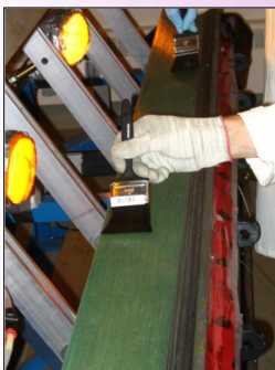
Each layer of the matrix consists of two layers of optical epoxy, one layer of fibres, and one sheet of lead.
