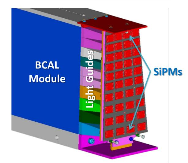
The BCAL modules are coupled on both ends to arrays of Silicon Photon Multipliers (SiPM) with light guides.
