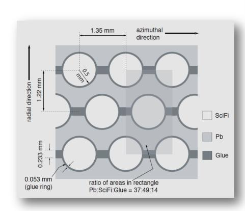
BCAL uses a Pb/SciFi matrix design to have both a compact size and a very good energy resolution.
