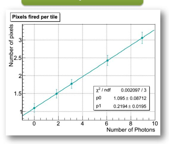
SiPM shows an excellent photon-counting capability and the pixels fired has a very linear dependence on the input light intensity.
