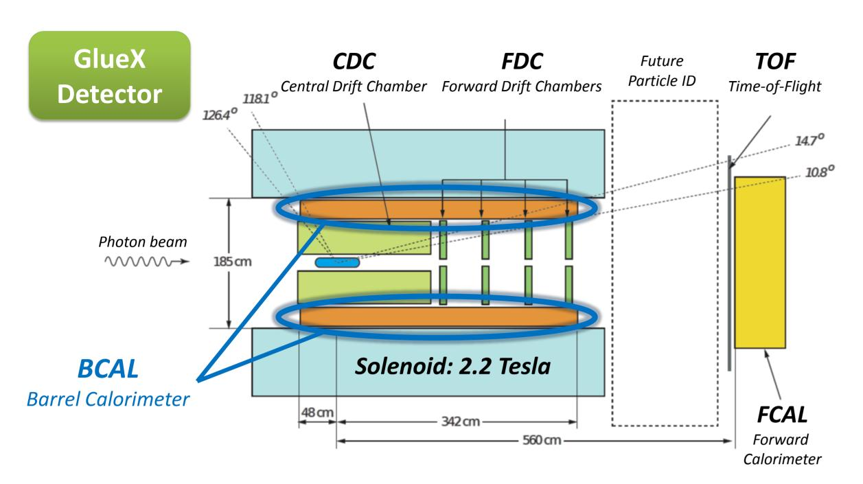
A 390 cm long Electromagnetic Barrel Calorimeter (BCAL) is inserted into the solenoid which generates a 2.2 Tesla magnetic field to detect particles in large angles. It measures energy deposition between 50 MeV to 5 GeV and provides timing and position information.
