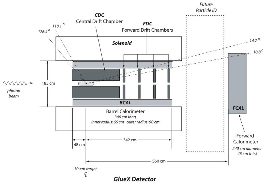
**Figure 1:** Simplified view of the GlueX detector: vertical cross-section along beam line. The tracking system is darkly shaded. Lightly shaded are the calorimeters. Not shown is the Start Counter around the target and the Time of Flight wall in front of the FCAL.
