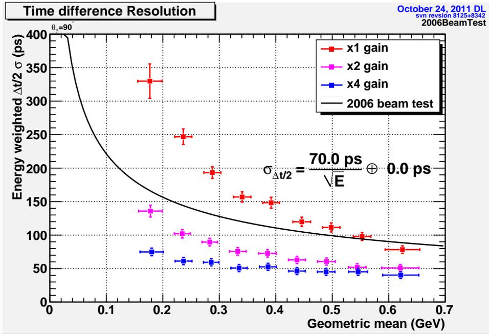
Figure 4: Time difference resolution ( $\Delta t/2$ ) for fully reconstructed BCAL showers. The black curve represents the final resolution reported for the 2006 Beam Test data. The markers indicate the results from the current Monte Carlo study with various gain factors.
