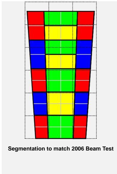
Figure 1: Segmentation used for the simulation study using the 2006 beam test configuration. The size and segmentation of the module in the 2006 test is shown by the dotted lines. The colored boxes indicate the segmentation used for the current study. In this picture, the beam enters from the center of the bottom edge.
