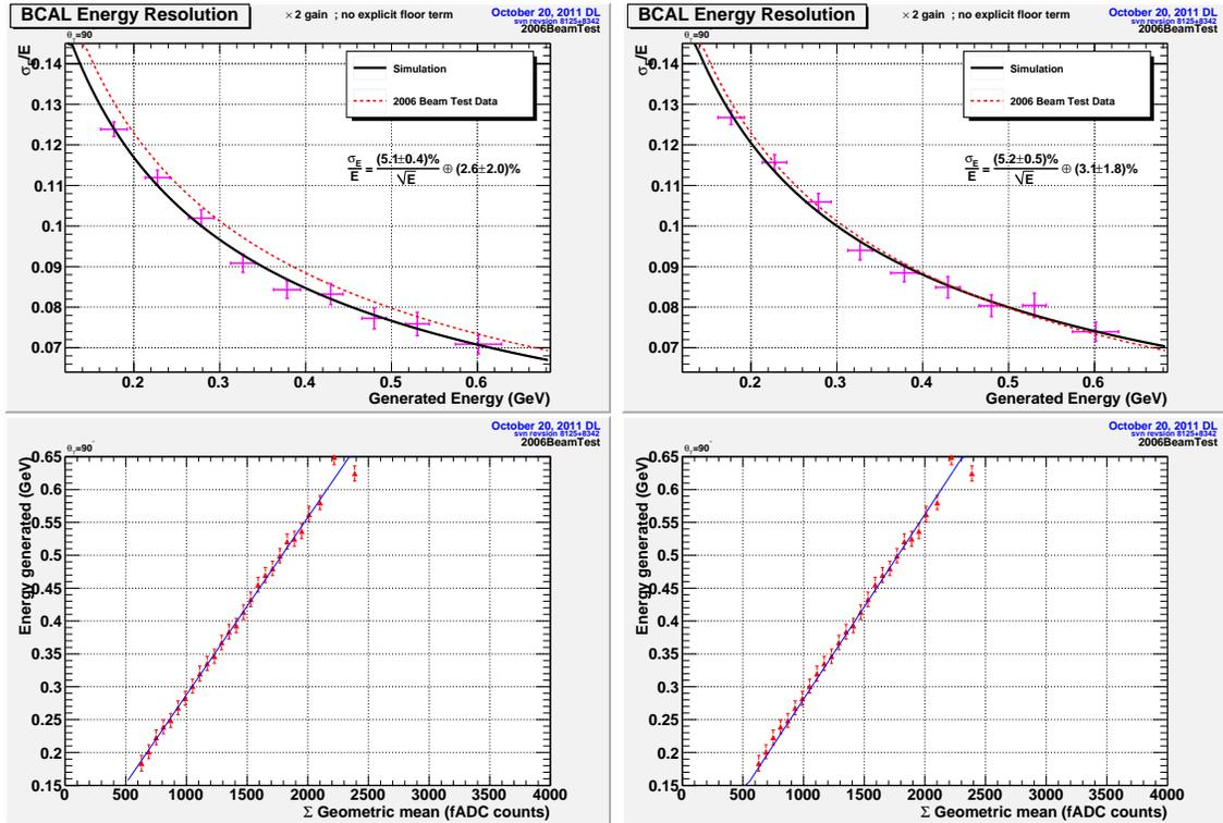
Figure 3: Energy resolution obtained from two different calibrations of the same dataset. The top two plots show the energy resolutions while the bottom two plots show the calibrations used to obtain the results. See text for more details.
