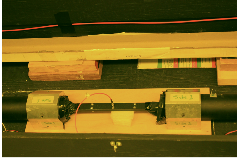
Figure 6.10: A picture of the FHLG in the dark box. SiPM is held at side 1 and the photodiode is held at side 2. (original in color)
