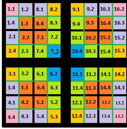
Figure 5.9: Schematic view of the SiPM's sub-cell families. (original in color)
