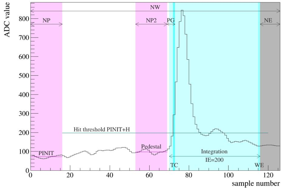
FIGURE 1. Examples of pulse analysis, showing the trigger, pedestal and hit search windows, and the integration region used with configuration parameter  $IE$  set to 30 (top) and 200 (bottom). Integration starts with the sample containing the leading edge of the pulse as determined by the timing algorithm.
