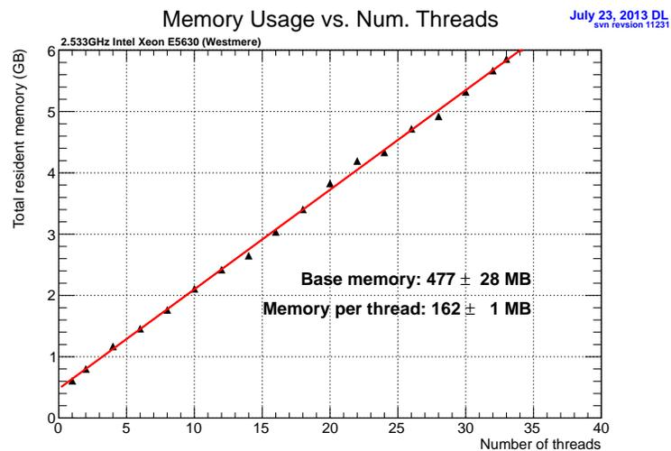
Figure 2: Memory usage vs. the number of threads for each of the 3 computers tested. The values of “Base Memory” and “Memory per thread” are the offset and slope of the linear fits shown. The total memory used by a single threaded process would be approximately the sum of these two numbers. This indicates memory usage by multi-threading rises at roughly 25% the rate that it does for multi-process.
