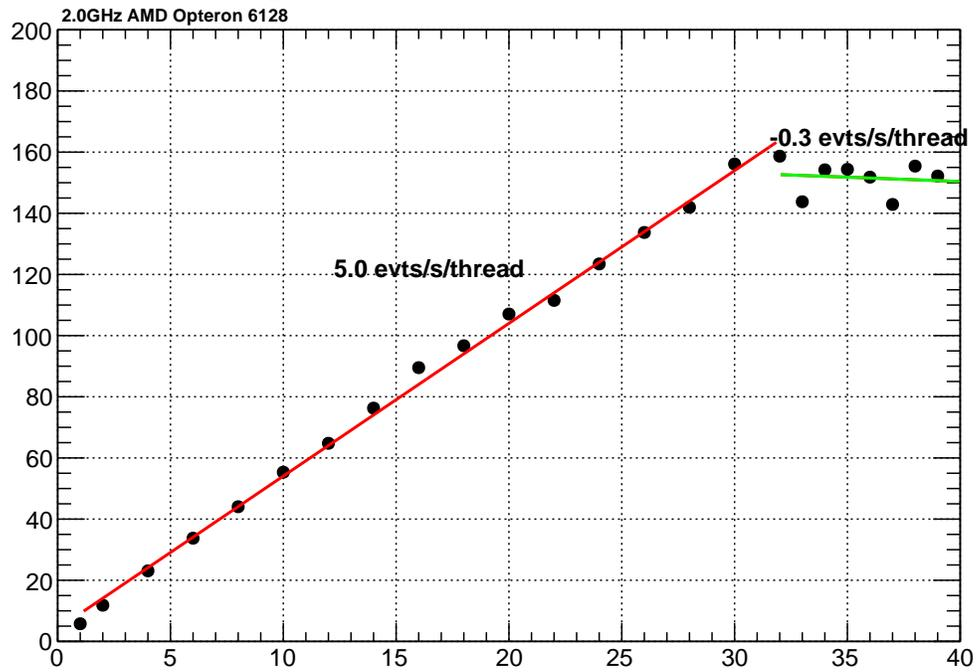
Figure 6: Event reconstruction rate vs. number of processing threads on a 32-core, 2.0GHz AMD Opteron computer. The green line is in the region where the processor is over-subscribed and no additional performance benefit is seen from the extra threads.
