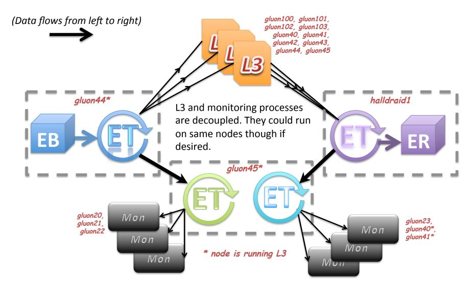
\*n.b. all L3 machines connected via InfiniBand
