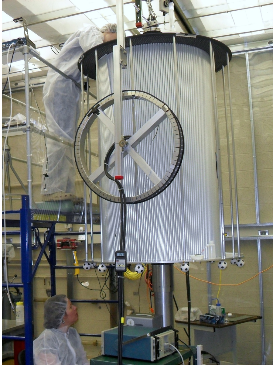
Figure 3.34: Wire tension measurement
