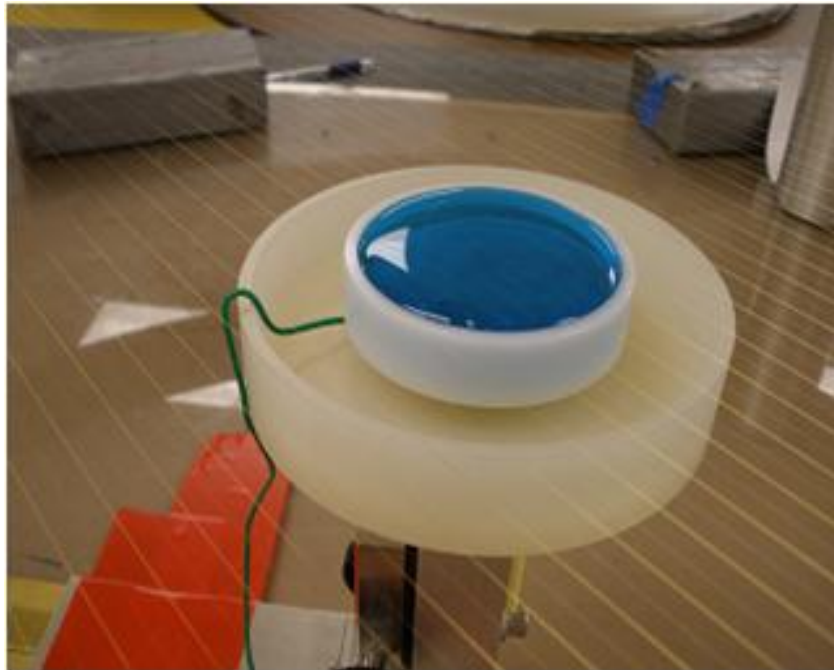
Figure 3.43: Wire deadening: a container filled with \text{CuSO}_4 is raised against the wires; voltage is applied between the sense wires and a copper electrode inside the container.
