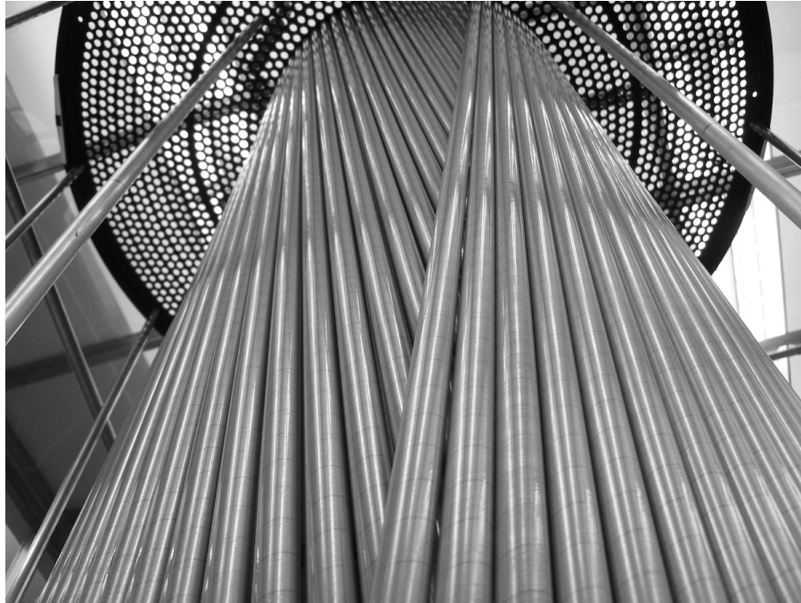
Figure 3.38: Straw tubes in stereo layers 8 and 9.
