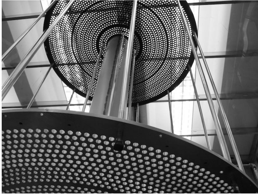
Figure 3.35: CDC frame prior to the installation of the straw tubes.
