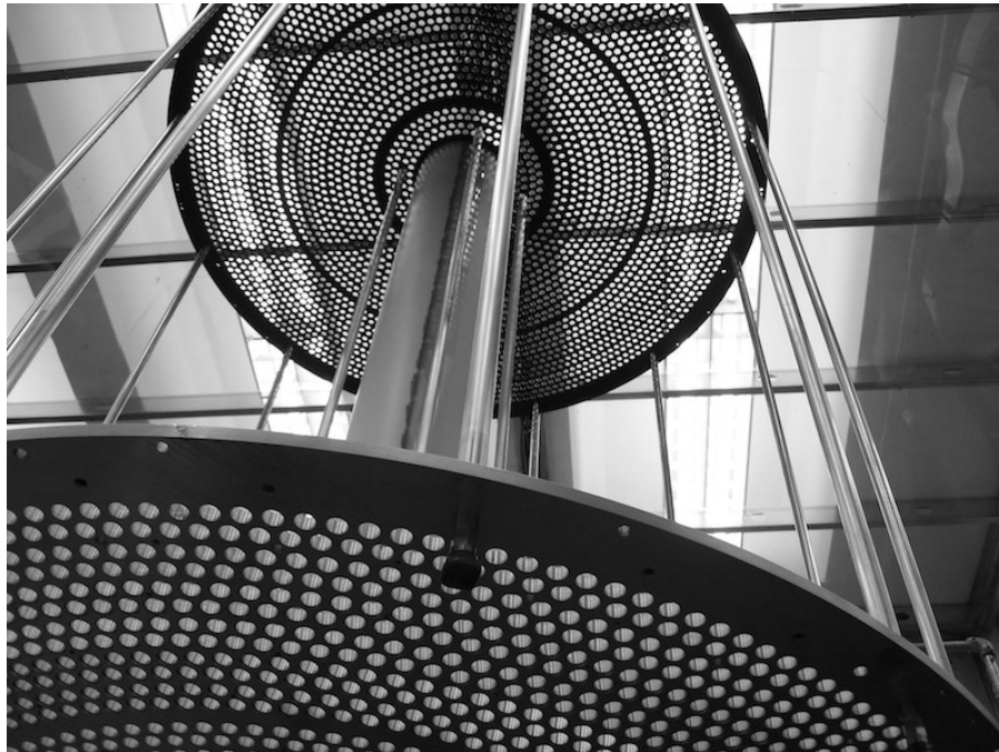
Figure 3.17: CDC frame prior to the installation of the straw tubes.
