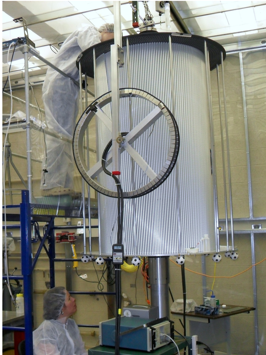
Figure 3.23: Wire tension measurement
