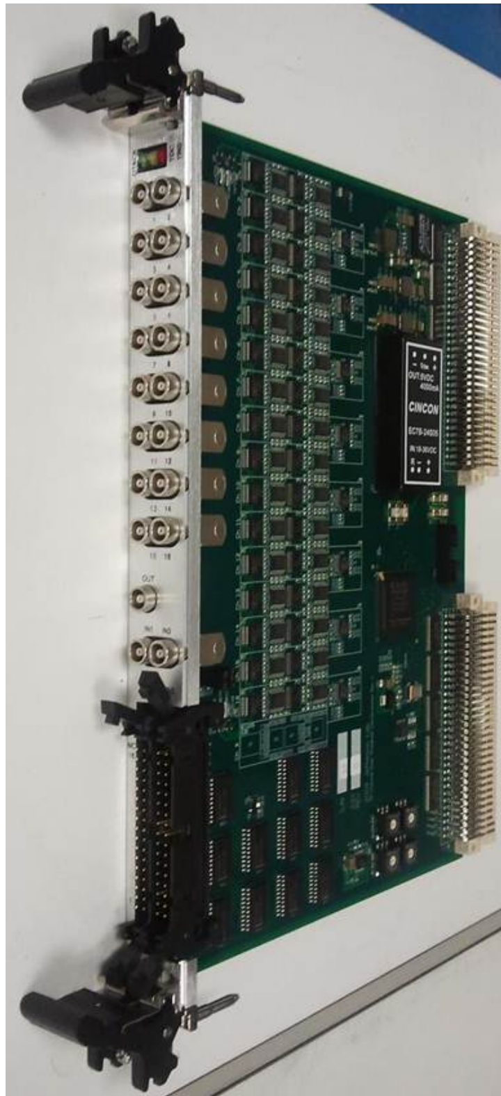
Figure 3.73: The JLab 16-ch discriminator
