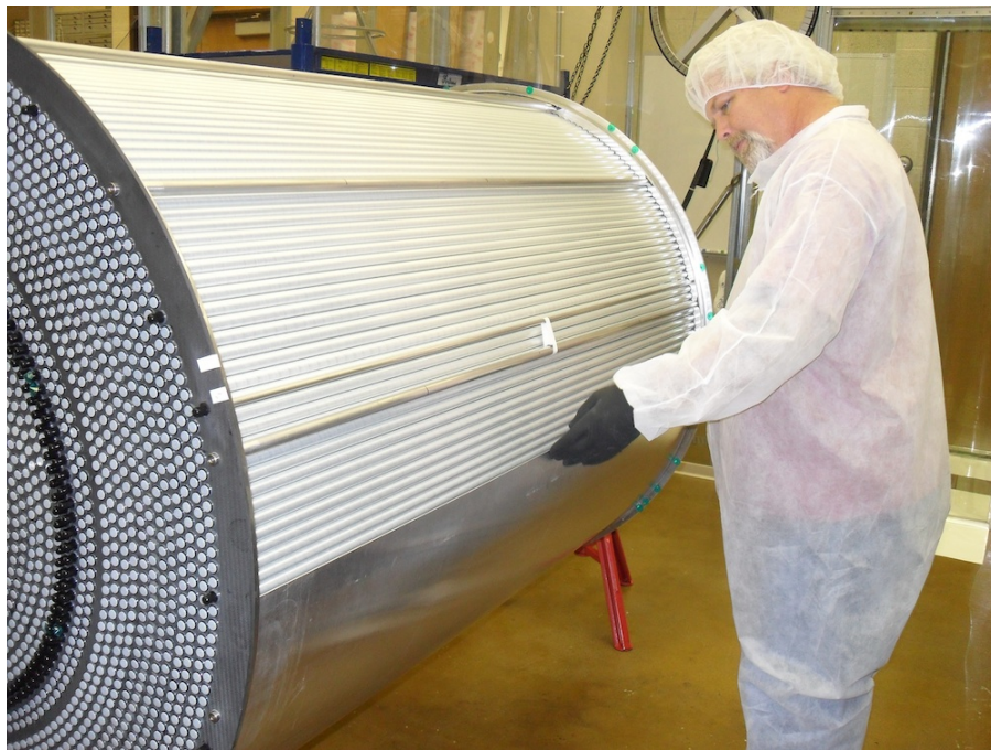
Figure 3.21: Straw tubes in layer 28, with one half of the outer shell in place.
