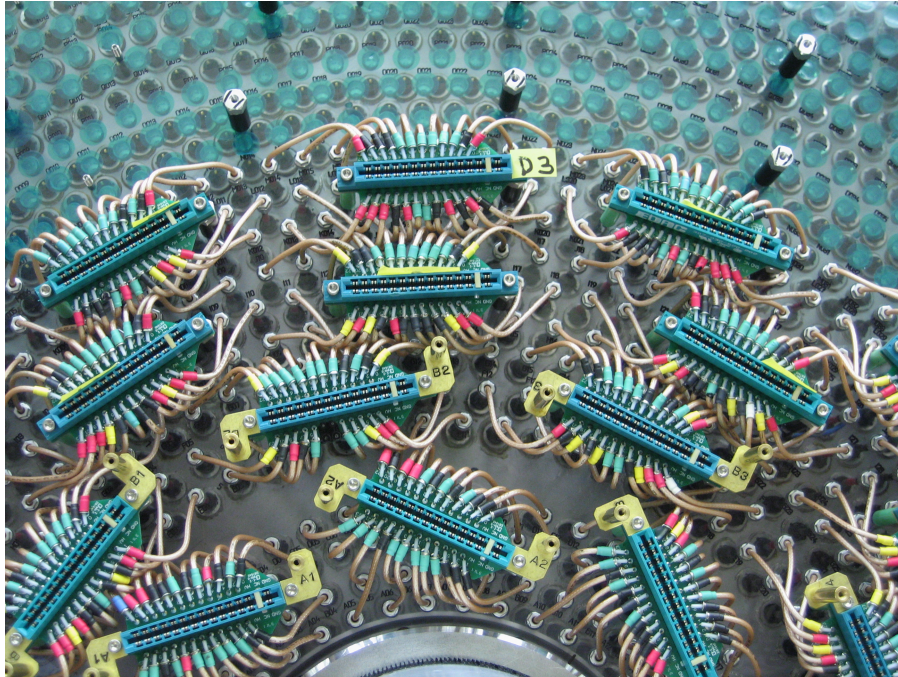
Figure 3.25: Hookup wires and transition boards.
