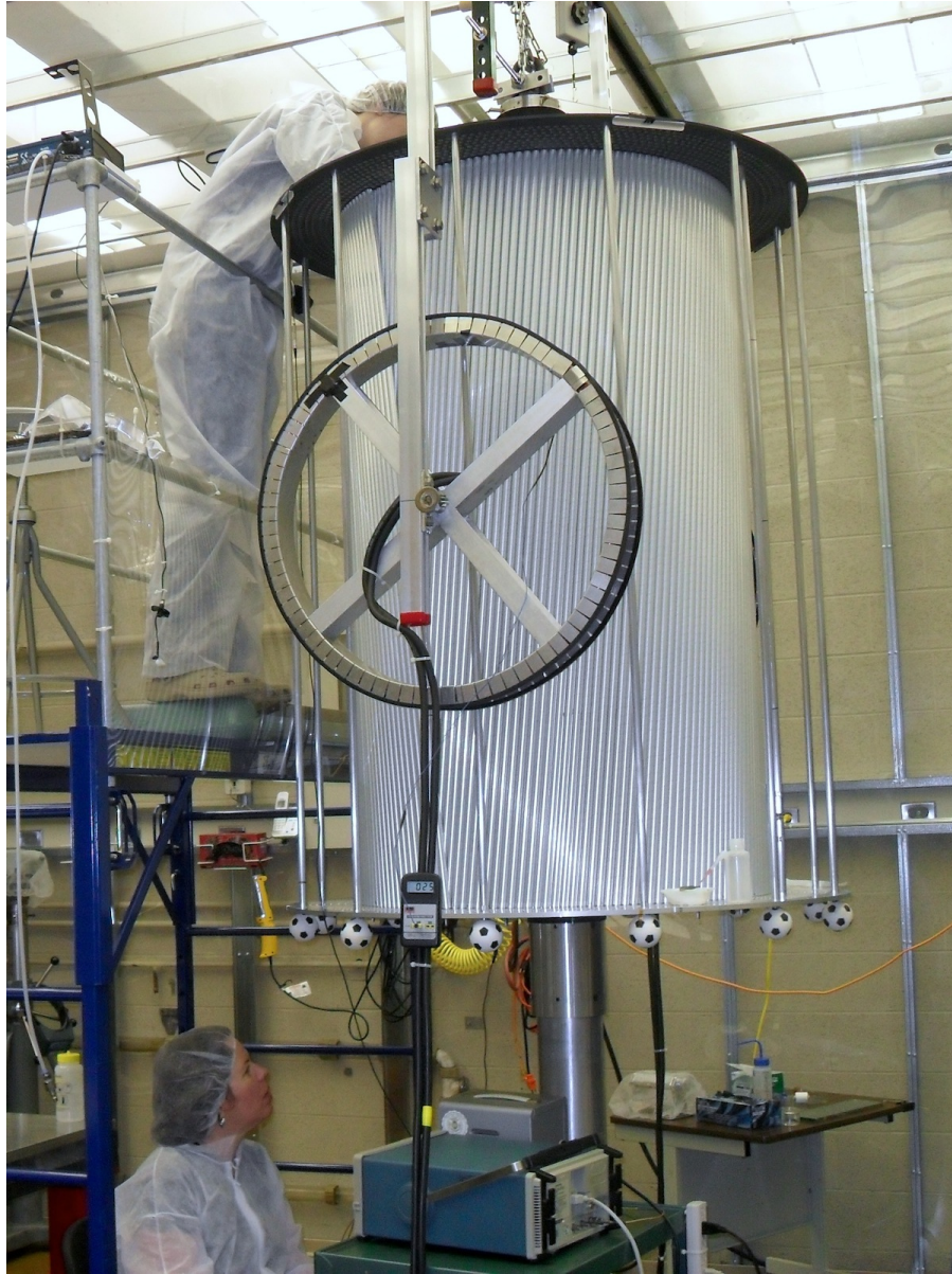
Figure 3.42: Wire tension measurement
