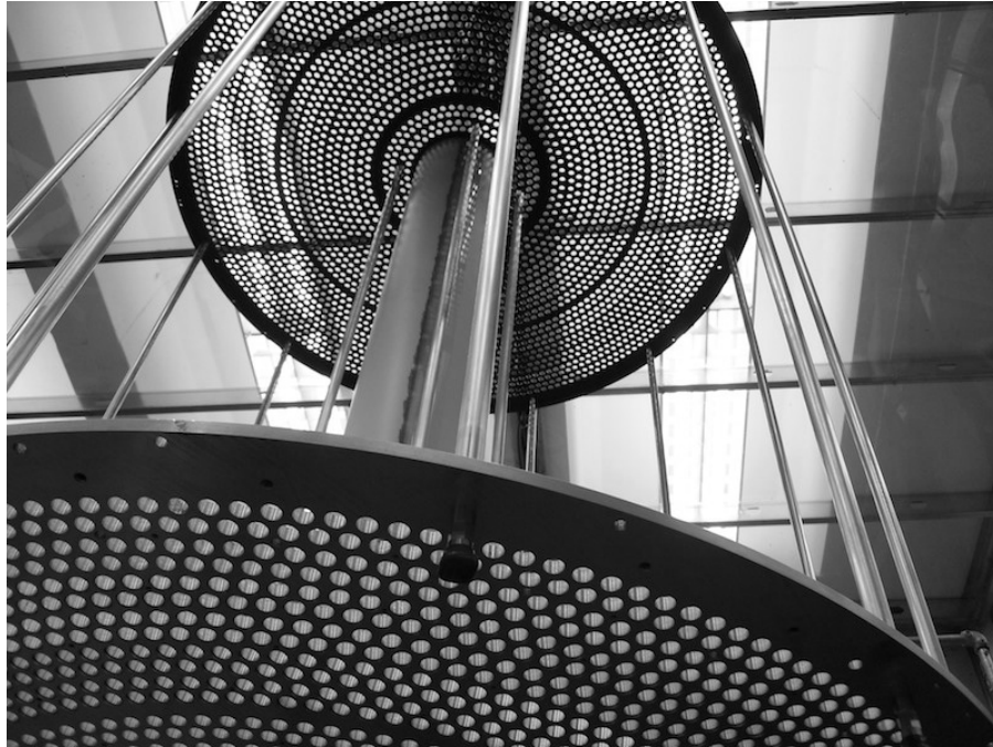
Figure 3.36: CDC frame prior to the installation of the straw tubes.
