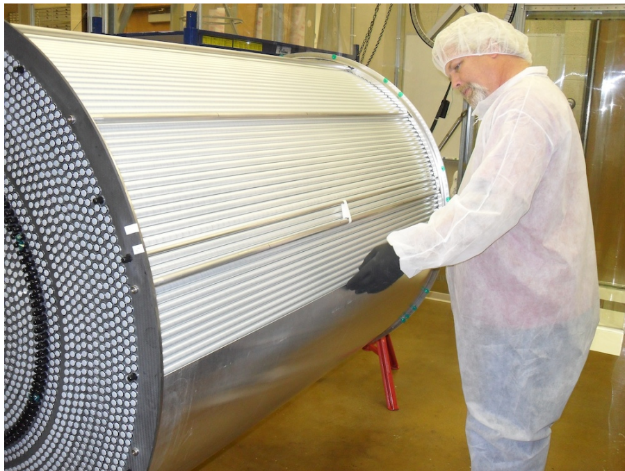
Figure 3.40: Straw tubes in layer 28, with one half of the outer shell in place.
