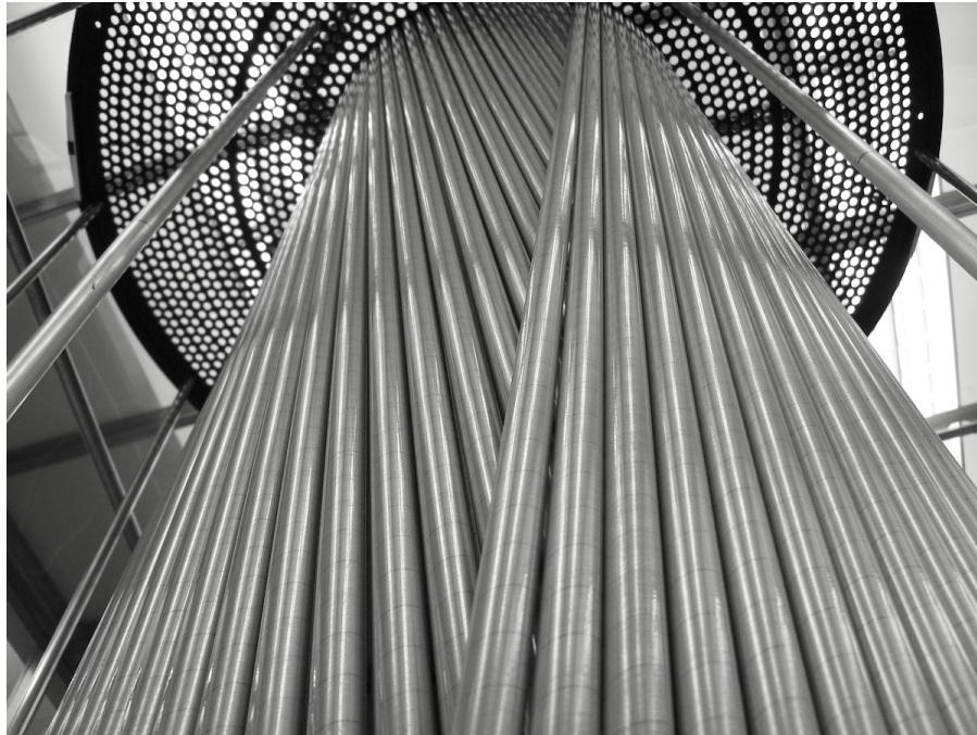
Figure 3.39: Straw tubes in stereo layers 8 and 9.
