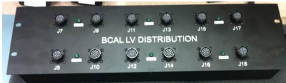
Figure 3.96: LV distribution chassis
