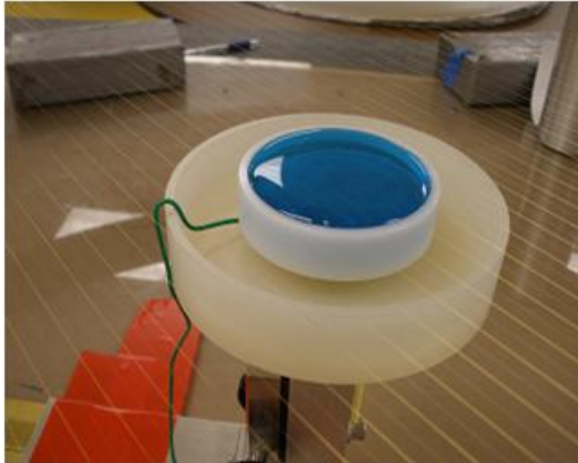
Figure 3.51: Wire deadening: a container filled with \text{CuSO}_4 is raised against the wires; voltage is applied between the sense wires and a copper electrode inside the container.
