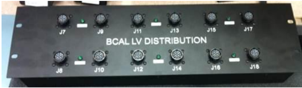
Figure 28: LV distribution chassis
