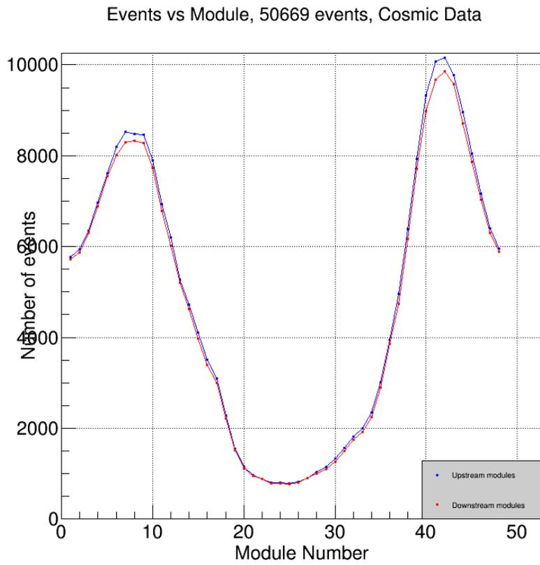
Figure 1: A tandem cosmic run, showing the amount of hits over the whole run for each module. Blue is for downstream, red is for upstream.
