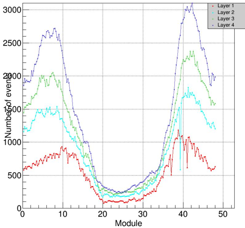
Figure 2: A tandem cosmic run, showing the amount of hits over the whole run for each layer (downstream).
