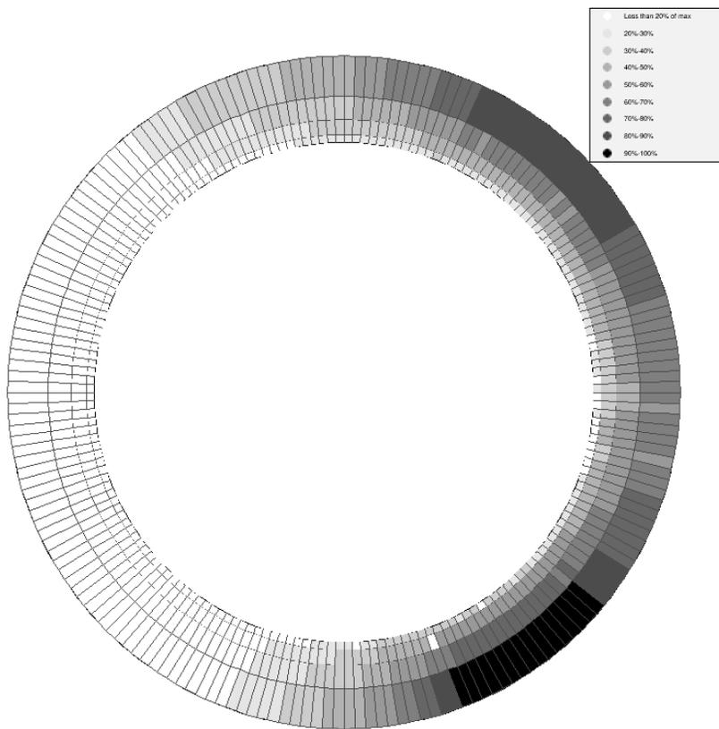
Figure 3: A tandem cosmic run, showing the amount of hits over the whole run for each channel. Darker regions correspond to more active regions. The north side is on the right, south is on the left. Modules begin at 3 o'clock and increase counter-clockwise.
