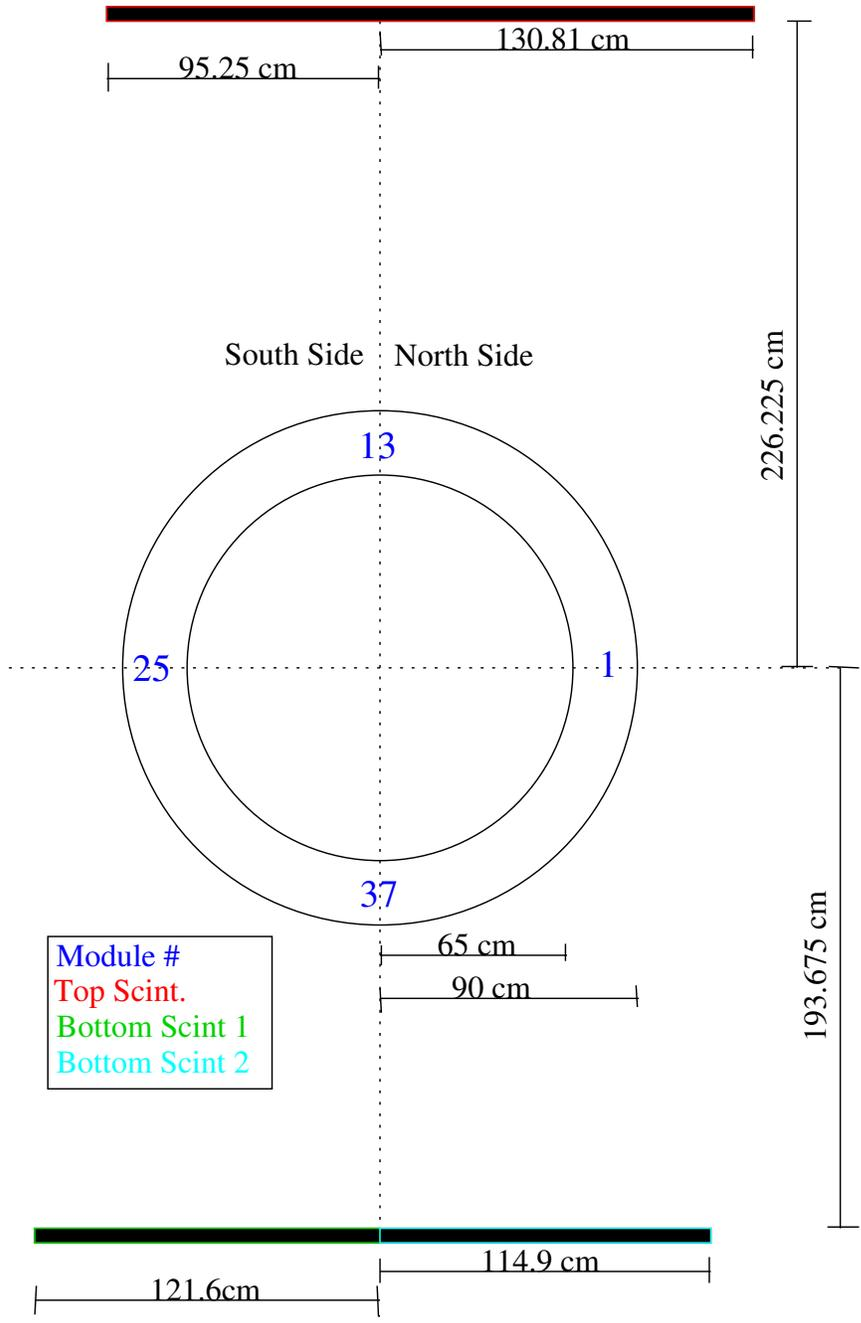
Figure 4: A to-scale drawing of the geometry of the BCAL. All measurements are in cm.
