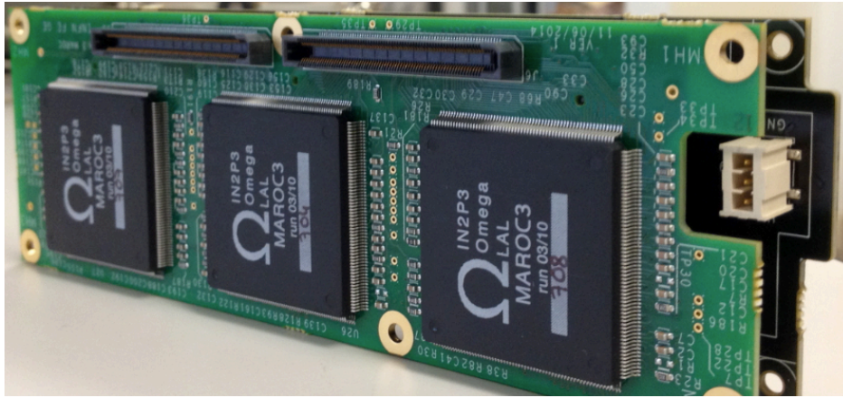
FIG. 38. ASIC board produced for the RICH detector for CLAS12 with MAROC chips installed [55].
