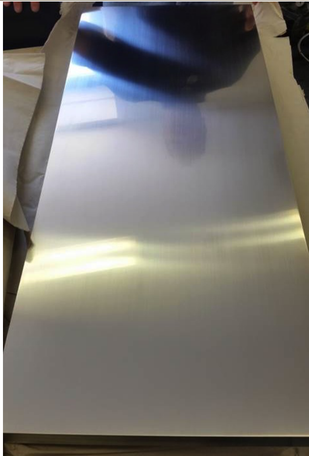
FIG. 27. Large flat mirror (1.1 m long) machined aluminum backing prototype.
