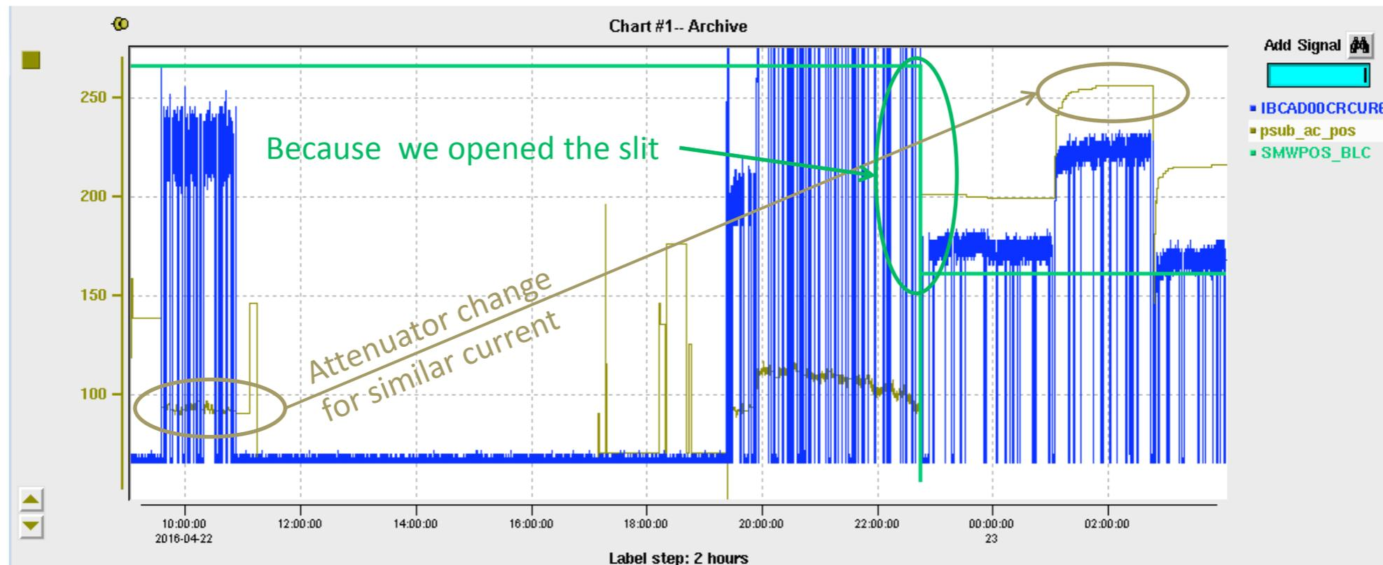
The laser attenuator setting (gold) in the Injector is a rough measure of the beam current at the very beginning of the machine. Ops opened the slit (green) probably because they were running out of room on the attenuator. That changed the attenuator setting drastically and stopped the beam from scrapping on the slit. The reduction of scraping on the slit is what helped stabilize the current.
