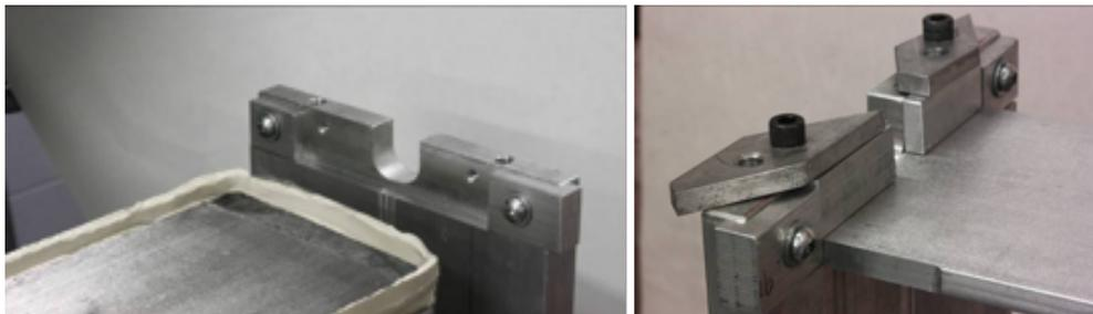
Figure 8: The white-tape dam built to hold the industrial epoxy for the top plate is shown on the left panel. The fixed stops which held the top plate motionless while the epoxy was curing, are shown on the right panel. (Color online)
