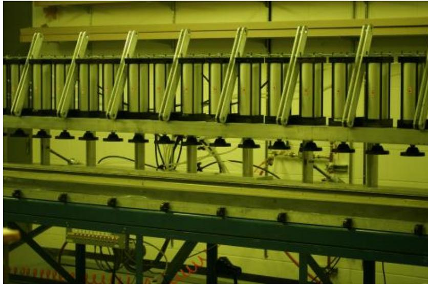
Figure 6: One of the electropneumatic presses is shown, with the aluminum connector arms and piston rams in the upright position. The press table is clearly seen as is the electronic control system in the lower left of the photograph. (Color online)
