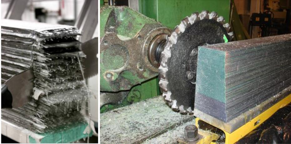
Figure 9: *Left panel:* A photograph of the end of a module after the completion of its build, showing the sawing of the excess length. *Right panel:* This photograph shows the machining of a prototype BCAL module. The cutter is clearly visible. Each set of four cutter blades was followed by a fifth, “wiper” blade, which removed excess lead so as to avoid scarring the lead-fiber surface. (Color online)
