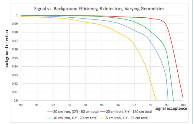
Compare blue (xy-iron-xy...) and green (x-iron-y-iron...): Green is better. To do: adjust so total amount of iron is identical.
