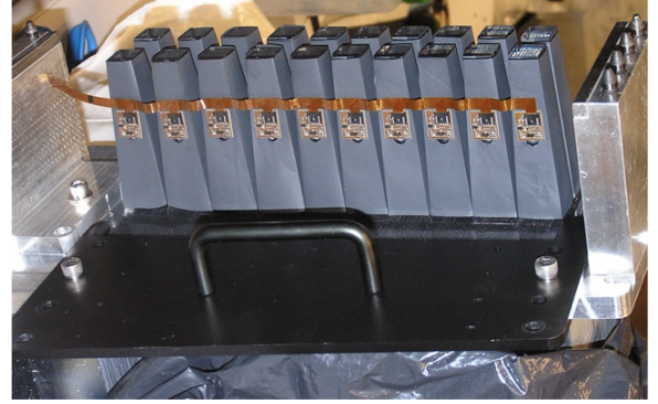
Figure 3.2: One end of a prototype BCAL module, showing two of its four sectors of light guides. The LED pulsers are mounted on the side of the light guides attached to a common flexible cable. The free end of the flexible cable connects to its control board (shown in Fig. 3.1) [38].
