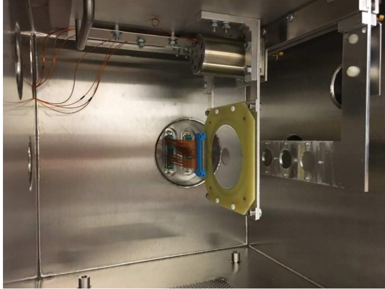
Figure 2.5: A picture of the triplet polarimeter detector. The beam enters from the right, some of the photons interact with electrons in the beryllium foil, and the beam proceeds into the experimental hall. The silicon strip detector (the doughnut-shape in the middle right of the photo) detects the recoil electron while the e^+e^- pair is detected by the Pair Spectrometer.
