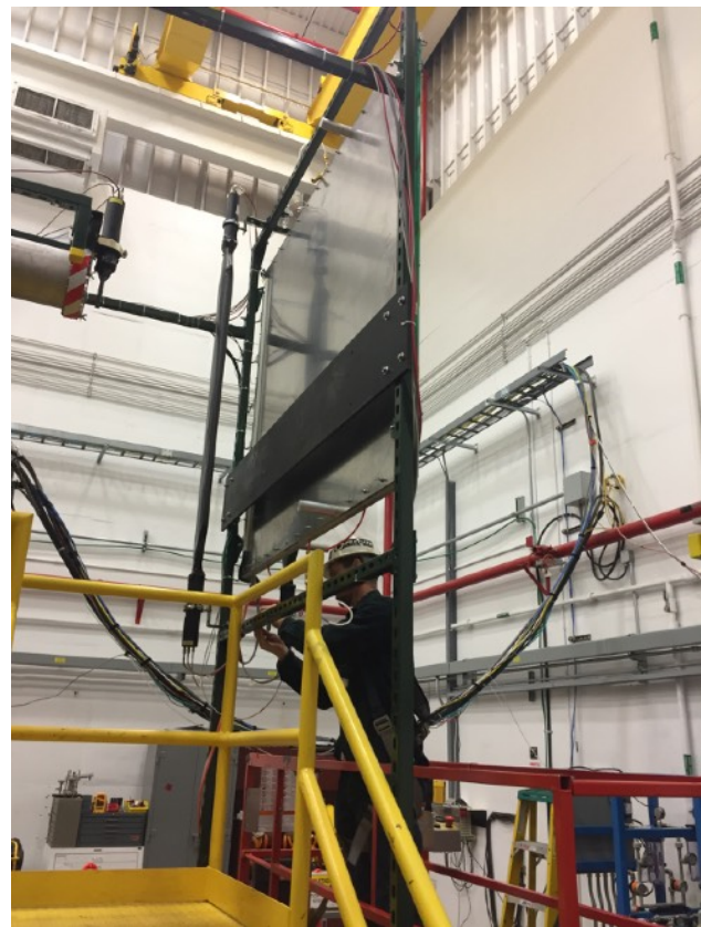
Fig. 2.1 Full-scale prototype MWPC mounted on the platform behind FCAL for a beam test.
