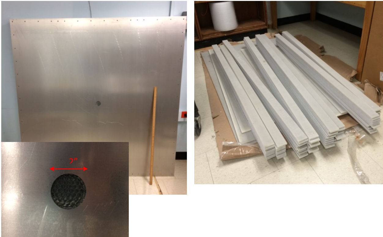
Fig. 3.2. Left, photo of honeycomb plate, with closeup photo of the central hole. Right, the G10 slats as they came from the supplier prior to machining at UMass.
